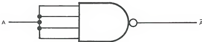
Fig. 30-20 Construction of NOT Circuit for NAND Gate
