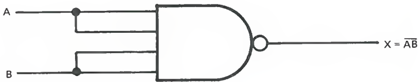
Fig. 30-19 Pairing Inputs to NAND Gate
