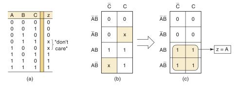
Here the output z is not specified as either 0 or 1 for the conditions A, B, C = 1, 0, 0 and A, B, C = 0, 1, 1. Instead, an x is shown for these conditions. The x represents the **don't-care condition**. A don't-care condition can come about for several reasons, the most common being that in some situations certain input combinations can never occur, and so there is no specified output for these conditions.
