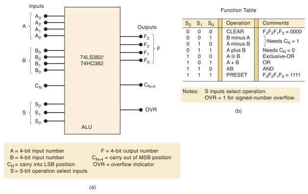
**FIGURE 6-15** (a) Block symbol for 74LS382/HC382 ALU chip; (b) function table showing how select inputs (*S*) determine what operation is to be performed on *A* and *B* inputs.
