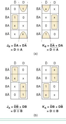
A and the desired NEXT state, along with the levels at each J and K input needed to achieve the transitions. Note that in all cases, the Direction input, D, does not change in going from the PRESENT to the NEXT state because it is an independent input that is held HIGH or LOW as the counter goes through its sequence.
