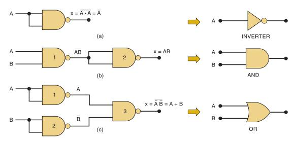
FIGURE 3-29 NAND gates can be used to implement any Boolean function.
