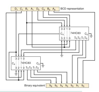
four-bit parallel adders can be wired to perform the conversion. This is one of several possible adder arrangements that will work. You may want to review the operation of this IC in Section 6-14.
