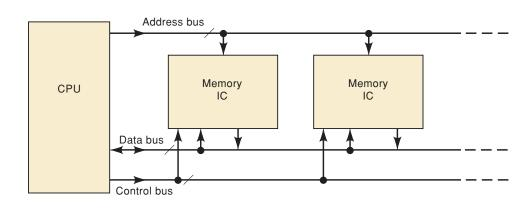
When a computer is executing a program of instructions, the CPU continually fetches (reads) information from those locations in memory that contain (1) the program codes representing the operations to be performed and (2) the data to be operated upon. The CPU will also store (write) data into memory locations as dictated by the program instructions. Whenever the CPU wants to write data to a particular memory location, the following steps must occur:
