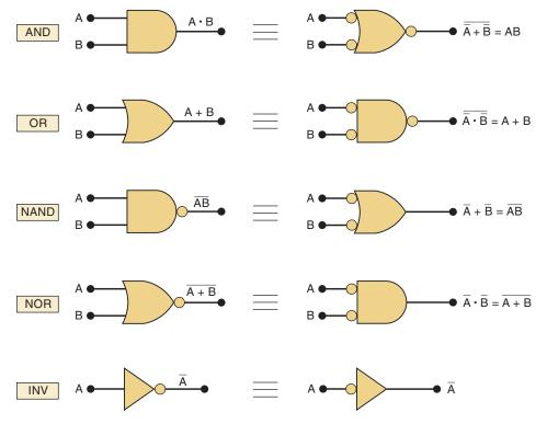
For example, the standard NAND symbol is an AND symbol with a bubble on its output. Following the steps outlined above, remove the bubble from the output, and add a bubble to each input. Then change the AND symbol to an OR symbol. The result is an OR symbol with bubbles on its inputs.
