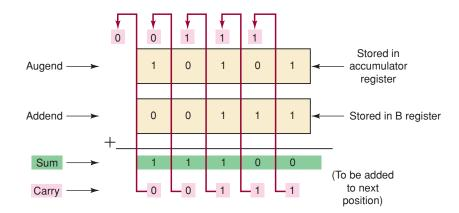
This carry must be added to the next position along with the augend and addend bits in that position. Thus, in the second position, 1 + 0 + 1 = 10, which is again a sum of 0 and a carry of 1. This carry is added to the next position together with the augend and addend bits in that position, and so on, for the remaining positions, as shown in Figure 6-5.
