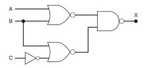
**B** 3-20. Determine the truth table for the circuit of Figure 3-24.
