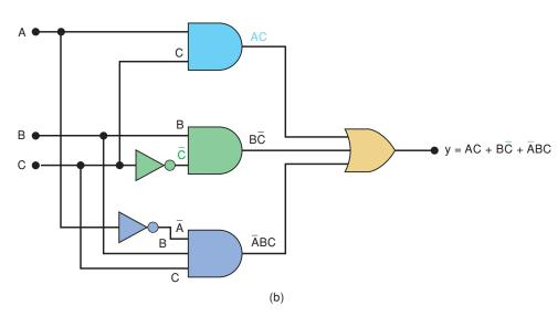
Each OR gate input is an AND product term, which means that an AND gate with appropriate inputs can be used to generate each of these terms. This is shown in Figure 3-17(b), which is the final circuit diagram. Note the use of INVERTERs to produce the  $\overline{A}$  and  $\overline{C}$  terms required in the expression.
