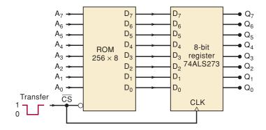
C, D 12-12. Repeat Problem 12-11 if the address inputs are changed 70 ns prior to the TRANSFER pulse.
