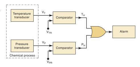
Since we want the alarm to be activated when either temperature *or* pressure is too high, it should be apparent that the two comparator outputs can be fed to a two-input OR gate. The OR gate output thus goes HIGH (1) for either alarm condition and will activate the alarm. This same idea can obviously be extended to situations with more than two process variables.
