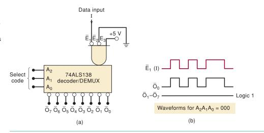
Figure 9-30(b) shows typical waveforms for the case where  $A_2A_1A_0=000$  selects output  $\overline{O}_0$ . For this case, the data signal applied to  $\overline{E}_1$  will be transmitted to  $\overline{O}_0$ , and all other outputs will remain in their inactive HIGH state.
