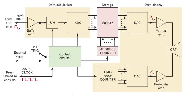
**FIGURE 11-26** Block diagram of a digital storage oscilloscope.
