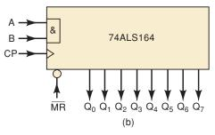
FIGURE 7-68 (a) Logic diagram for the 74ALS164; (b) logic symbol.
