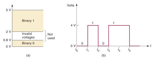
**FIGURE 1-8** (a) Typical voltage assignments in digital system; (b) typical digital signal timing diagram.
