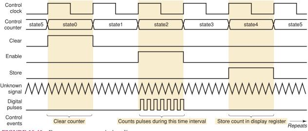
FIGURE 10-40 Frequency counter timing diagram.
