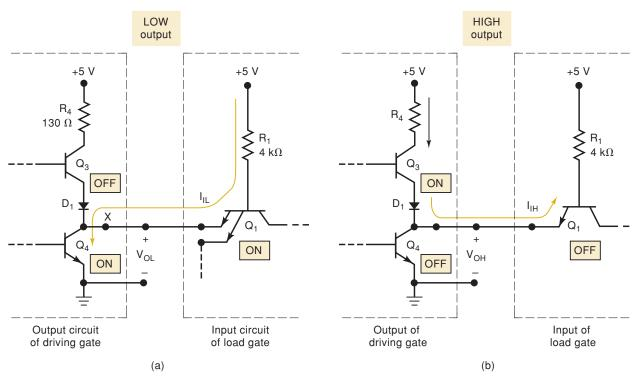
**FIGURE 8-9** (a) When the TTL output is in the LOW state,  $Q_4$  acts as a current sink, deriving its current from the load. (b) In the output HIGH state,  $Q_3$  acts as a current source, providing current to the load gate.
