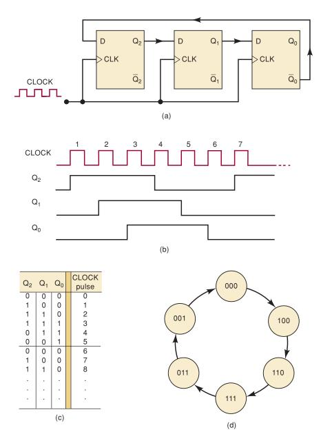
Figure 7-72, the result is a MOD-10 Johnson counter, where each FF output waveform is a square wave at one-tenth the clock frequency. Thus, it is possible to construct a MOD-N counter (where N is an even number) by connecting N/2 flip-flops in a Johnson-counter arrangement.
