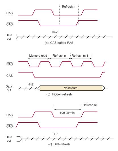
However, if this will slow the program execution down too much, it may require some distributed refreshing using  $\overline{CAS}$ -before- $\overline{RAS}$  or hidden refresh cycles. In any case, all cells must be refreshed within the allotted time or data will be lost.
