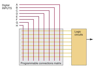
configure these devices by placing 1s and 0s in a grid manually (which is how they did it back in the 1970s).
