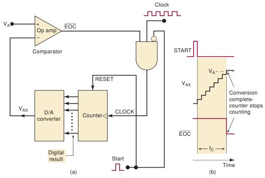
FIGURE 11-13 Digital-ramp ADC.
