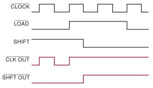
4-43. Possible faults: faulty  $V_{CC}$  or ground on Z2; Z2-1 or Z2-2 open internally or externally; Z2-3 internally open
