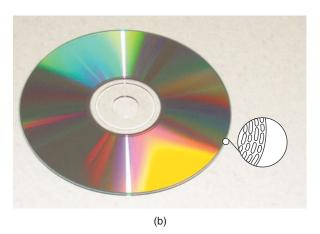
Another example is shown in Figure 1-7(b), where binary numbers are stored on a CD. The inner surface (under a transparent plastic layer) is coated with a highly reflective aluminum layer. Holes are burned through this reflective coating to form "pits" that do not reflect light the same as the unburned areas. The areas where the pits are burned are considered "1" and the reflective areas are "0."
