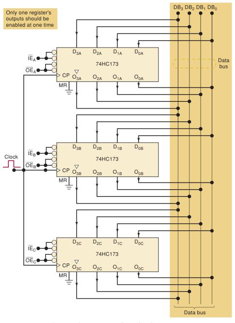
**FIGURE 9-44** Tristate registers connected to a data bus.
