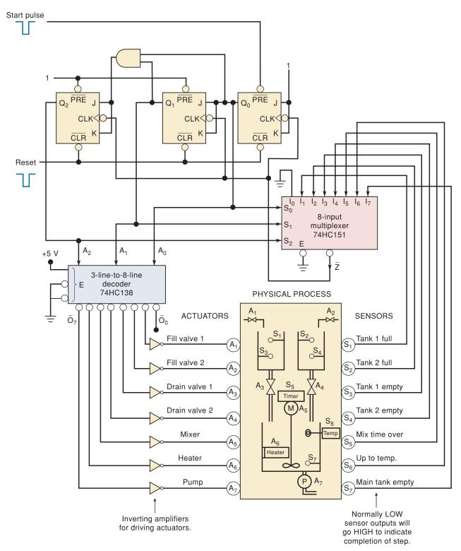
FIGURE 9-26 Seven-step control sequencer.
