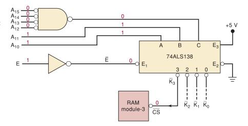
The x's under  $A_9$  through  $A_0$  indicate don't care because these address lines are not used by the decoder to select module-3.  $A_9$  to  $A_0$  can be any combination ranging from 0000000000 to 11111111111, depending on which word in module-3 is being accessed. Thus, the complete range of addresses for module-3 is determined by using all 0s, and then all 1s for the x's.
