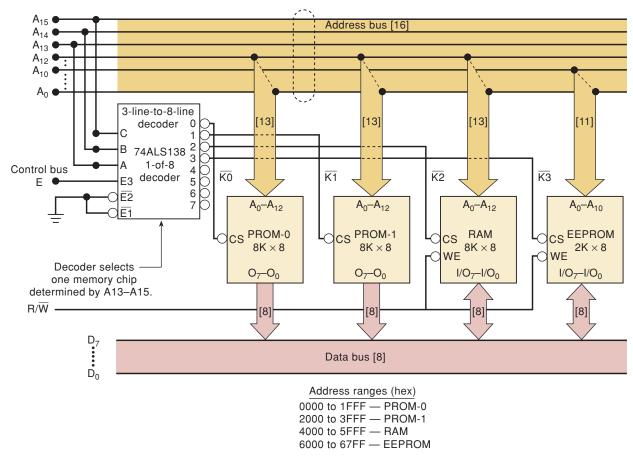
**FIGURE 12-38** A system with incomplete address decoding.
