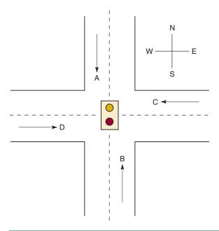
outputs are LOW (0) when no vehicle is present and HIGH (1) when a vehicle is present. The intersection traffic light is to be controlled according to the following logic:
