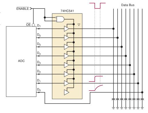
**FIGURE 9-48** Simplified representation of bus arrangement.
