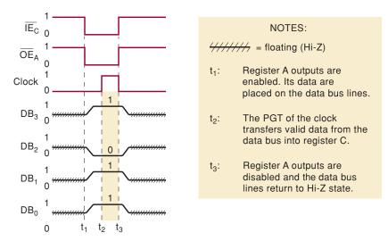
to stabilize on the bus, the PGT of the clock is applied at  $t_2$ . This PGT will transfer these logic levels into register C because  $\overline{IE}_C$  is active. If the PGT occurs before the data bus has valid logic levels, unpredictable data will be transferred into C.
