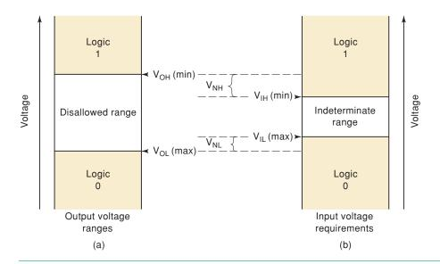
and it is the difference between the largest possible LOW output and the maximum input voltage required for a LOW. When a LOW logic output is driving a logic input, any positive noise spikes greater than  $V_{\rm NL}$  can cause the voltage to rise into the indeterminate range.
