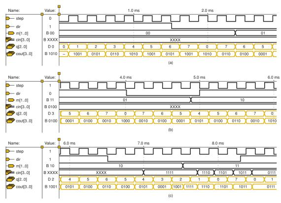
FIGURE 10-10 Simulation testing of the complete stepper driver.
