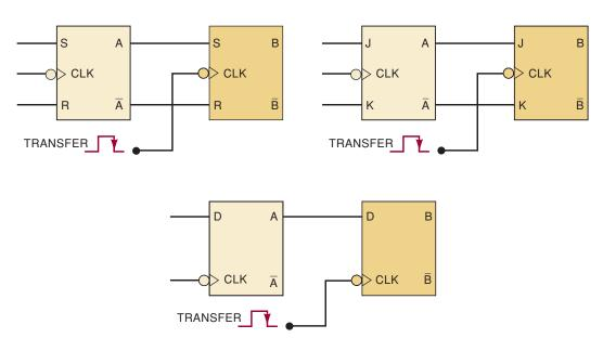
**FIGURE 5-42** Synchronous data transfer operation performed by various types of clocked FFs.
