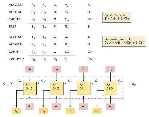
FIGURE 6-19 Four-bit parallel adder.
