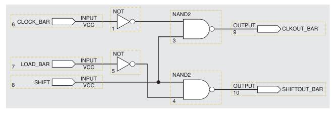
FIGURE 4-33 Logic diagram using schematic capture.
