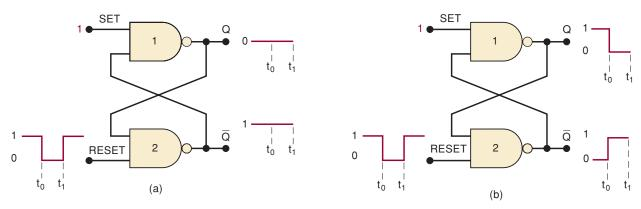
**FIGURE 5-5** Pulsing the RESET input to the LOW state when (a) Q = 0 prior to RESET pulse; (b) Q = 1 prior to RESET pulse. In each case, Q ends up LOW.
