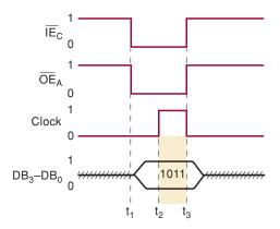
ital systems, usually the 8-, 16-, or 32-line data buses. These larger buses generally have many more than three devices tied to the bus, but the basic data transfer operation is the same: one device has its outputs enabled so that its data are placed on the data bus; another device has its inputs enabled so that it can take these data off the bus and latch them into its internal circuitry on the appropriate clock edge.
