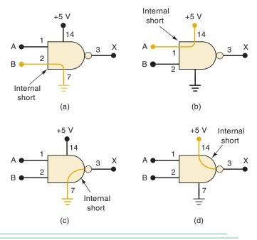
Similarly, an IC input pin could be internally shorted to +5 V, as in Figure 4-35(b). This would keep that pin stuck in the HIGH state. If this input pin is being driven by a logic signal A, it will effectively short A to +5 V.
