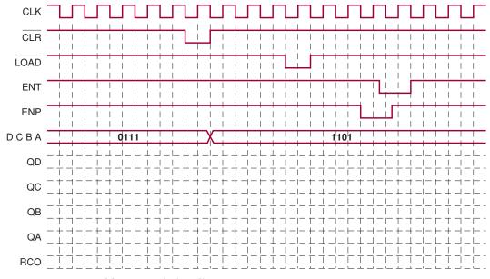
FIGURE 7-96 Problem 7-17 timing diagram.
