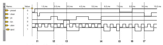
FIGURE 5-69 Simulation of the JK flip-flop.
