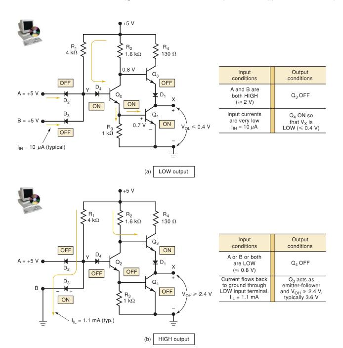
FIGURE 8-8 TTL NAND gate in its two output states.
