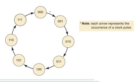
Each circle represents one possible state, as indicated by the binary number inside the circle. For example, the circle containing the number 100 represents the 100 state (i.e.,  $Q_2 = 1$ ,  $Q_1 = Q_0 = 0$ ).
