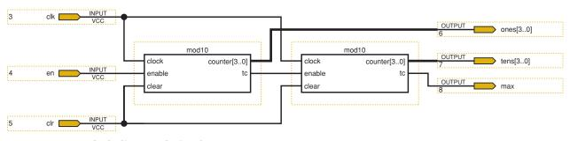
FIGURE 7-52 Block diagram design for a MOD-100 BCD counter.
