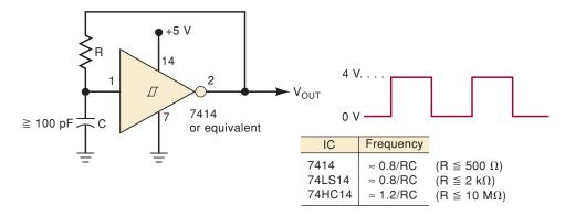
and *RC* values is shown in Figure 5-55 for three different Schmitt-trigger INVERTERs. Note the maximum limits on the resistance value for each device. The circuit will fail to oscillate if *R* is not kept below these limits.
