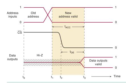
the address inputs are already set to their new values, but the ROM outputs have not yet been enabled. When  $\overline{CS}$  goes LOW to enable the outputs, the delay will be  $t_{\rm OE}$ .
