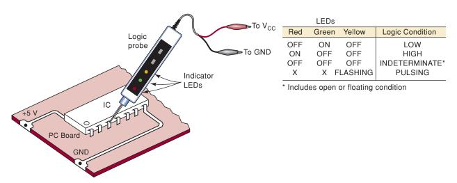
**FIGURE 4-34** A logic probe is used to monitor the logic level activity at an IC pin or any other accessible point in a logic circuit.
