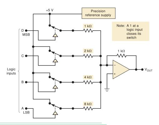
Each digital input controls a semiconductor switch such as the CMOS transmission gate we studied in Chapter 8. When the input is HIGH, the switch closes and connects a *precision reference supply* to the input resistor; when the input is LOW, the switch is open. The reference supply produces a very stable, precise voltage needed to generate an accurate analog output.
