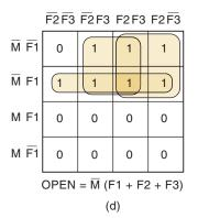
input is a 1 are don't-care conditions. We can place an *x* in the *OPEN* output column for those eight cases where more than one *F* input is 1.
