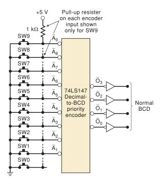
words, when the first key is depressed, the BCD code for that digit is sent to a four-bit FF register; when the second switch is depressed, the BCD code for that digit is sent to *another* four-bit FF register, and so on. Thus, a calculator that can handle eight digits will have eight four-bit registers to store the BCD codes for these digits. Each four-bit register drives a decoder/driver and a numerical display so that the eight-digit number can be displayed.
