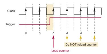
In order to know what the *trigger* was on the last active clock edge, the system must remember the last value that *the trigger had at that point*. This is done by storing the value of the trigger bit in a flip-flop. Recall that we discussed a similar concept in Chapter 5 when we talked about using a flip-flop to detect a sequence. The code for a one-shot is written so that the counter is loaded only after a rising edge is detected on the *trigger* input.
