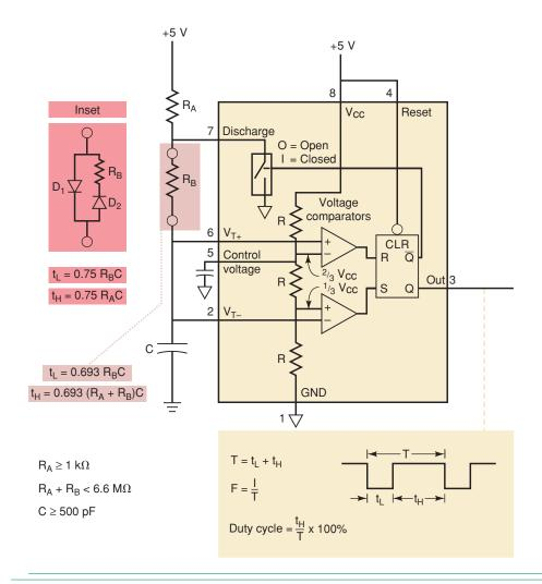
rectangular waveform that switches between two logic levels, with the time intervals at each logic level determined by the *R* and *C* values.
