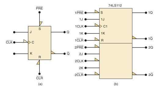
like the one symbolized in Figure 5-33(a). Note how the inputs and outputs are numbered. Also note that the input labels inside the rectangles are shown only for the top FF. It is understood that the inputs to the bottom FF are in the same arrangement as the top one. This same IC symbol applies to the CMOS 74HC112.
