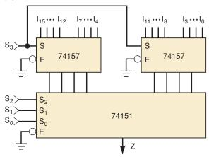
9-32. (b) The total number of connections in the circuit using MUXes is 63, not including  $V_{CC}$  and GND, and not including the connections to counter clock inputs. The total number for the circuit using separate decoder/drivers is 66.
