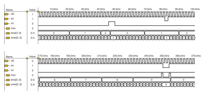
FIGURE 7-53 Simulation results for MOD-100 BCD counter design.
