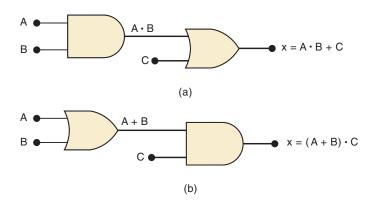
the circuit in Figure 3-13(a). This circuit has three inputs, A, B, and C, and a single output, x. Utilizing the Boolean expression for each gate, we can easily determine the expression for the output.
