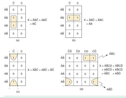
represents  $\overline{ABC}$ , and the second represents  $AB\overline{C}$ . Note that in these two terms only the A variable appears in both normal and complemented (inverted) form, while B and  $\overline{C}$  remain unchanged. These two terms can be looped (combined) to give a resultant that eliminates the A variable because it appears in both uncomplemented and complemented forms. This is easily proved as follows:
