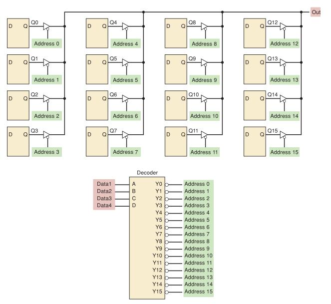
FIGURE 13-15 Functional block diagram for an LUT.
