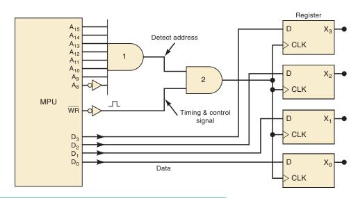
outputs  $A_{15}$ ,  $A_{14}$ ,  $A_{13}$ ,  $A_{12}$ ,  $A_{11}$ ,  $A_{10}$ ,  $A_{9}$ ,  $A_{8}$ . Most MPUs have at least 16 available address outputs, but they are not always all used. A second set of MPU outputs consists of the four *data lines*  $D_{3}$ ,  $D_{2}$ ,  $D_{1}$ ,  $D_{0}$ . Most MPUs have at least eight available data lines. The other MPU output is a timing control signal  $\overline{WR}$ , which goes LOW when the MPU is ready to write.
