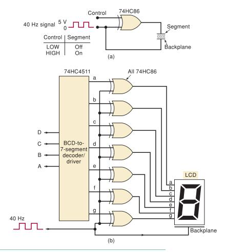
the backplane are equal. Because there is no difference in voltage, the segment will be OFF. When the CONTROL input is HIGH, the XOR output will be the INVERSE of the 40-Hz square wave, so that the signal applied to the segment is out of phase with the signal applied to the backplane. As a result, the segment voltage will alternately be at +5 V and at -5 V relative to the backplane. This ac voltage will turn ON the segment.
