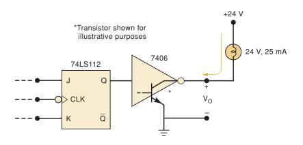
Q=0, the 7406 output transistor turns off; there is no path for current, and the lamp turns off. In this state, the full 24 V will appear across the OFF output transistor so that  $V_{\rm OH}=24$  V, which is lower than the 7406 maximum  $V_{\rm OH}$  rating.
