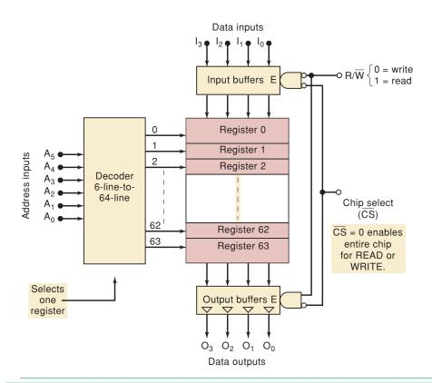
ranging from 0 to  $63_{10}$ . In order to select one of the 64 address locations for reading or writing, a binary address code is applied to a decoder circuit. Because  $64 = 2^6$ , the decoder requires a six-bit input code. Each address code activates one particular decoder output, which in turn enables its corresponding register. For example, assume an applied address code of
