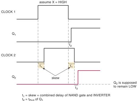
$t_2 = t_{PLH} \text{ of } Q_1$
