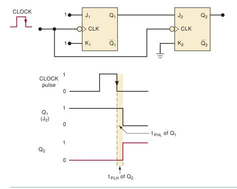
The potential timing problem is this: because  $Q_1$  will change on the NGT of the clock pulse, the  $J_2$  input of  $Q_2$  will be changing as it receives the same NGT. This could lead to an unpredictable response at  $Q_2$ .
