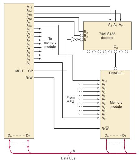
FIGURE 9-83 Basic microprocessor-to-memory interface circuit for Problem 9-63.
