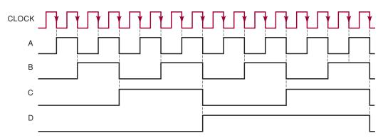
**FIGURE 7-2** Counter waveforms showing frequency division by 2 for each FF.
