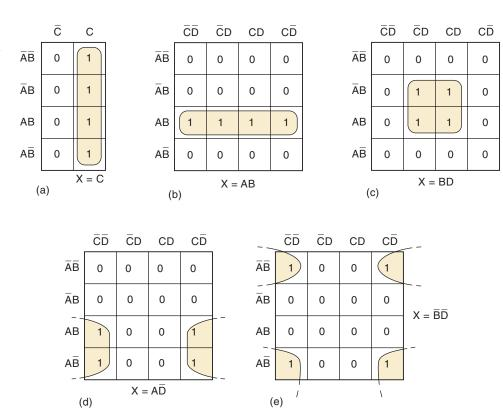
As another example, consider Figure 4-13(d), where the four squares containing 1s are  $AB\overline{C}\,\overline{D}$ ,  $A\,\overline{B}\,\overline{CD}$ ,  $ABC\overline{D}$ , and  $A\overline{B}C\overline{D}$ . Examination of these terms indicates that only the variables A and  $\overline{D}$  remain unchanged, so that the simplified expression for X is
