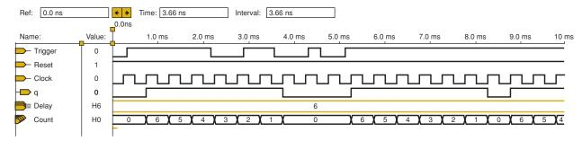
FIGURE 7-90 Simulation of the nonretriggerable one-shots.
