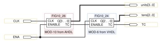
FIGURE 10-32 Graphically combining HDL blocks to make a MOD-60.
