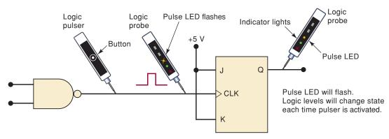
**FIGURE 8-53** A logic pulser can inject a pulse at any node that is not shorted directly to ground or  $V_{CC}$ .
