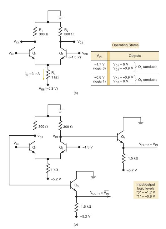
FIGURE 8-41 (a) Basic ECL circuit; (b) with addition of emitter followers.
