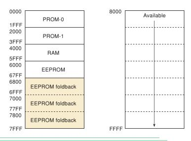
clearly shows the addresses that each device is assigned to as well as the memory space that is available for expansion.
