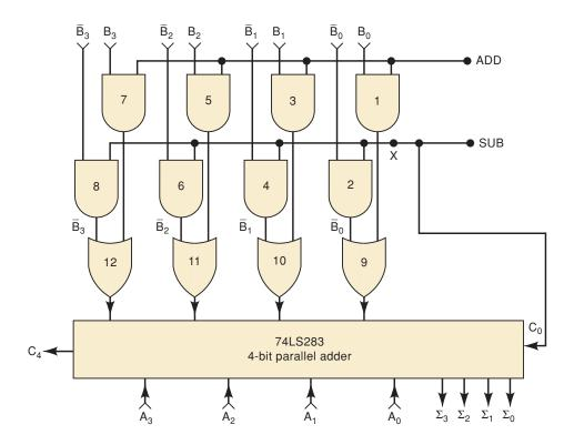
checks the connection between the SUB signal and the  $C_0$  input to the adder and finds that it is open due to a bad solder connection. This open connection explains the observed results because the TTL adder responds as if  $C_0$  were a constant logic 1, causing an extra 1 to be added to the result in modes 1 and 2. The open connection would have no effect on mode 3 because  $C_0$  is supposed to be a 1 anyway.
