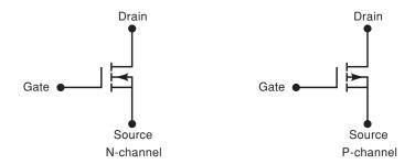
P- or N-channel. The symbols show a broken line between the *source* and the *drain* to indicate that there is *normally* no conducting channel between these electrodes. The symbol also shows a separation between the *gate* and the other terminals to indicate the very high resistance (typically around  $10^{12}~\Omega$ ) of the oxide layer between the gate and the channel, which is formed in the substrate.
