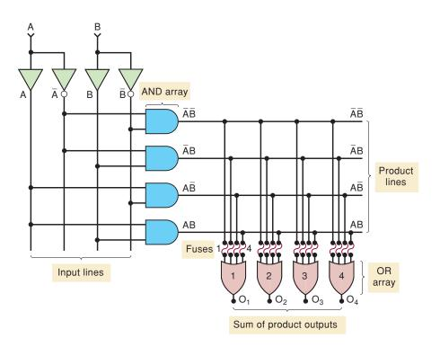
Each of the inputs *A* and *B* feed both a noninverting buffer and an inverting buffer to produce the true and inverted forms of each variable. These are the *input lines* to the AND gate array. Each AND gate is connected to two different input lines to generate a unique product of the input variables. The AND outputs are called the *product lines*.
