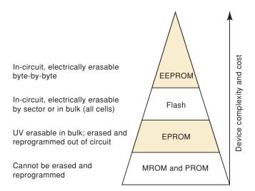
to 100  $\mu$ s for the most advanced EPROM and 5 ms for EEPROM (which includes automatic byte erase time).
