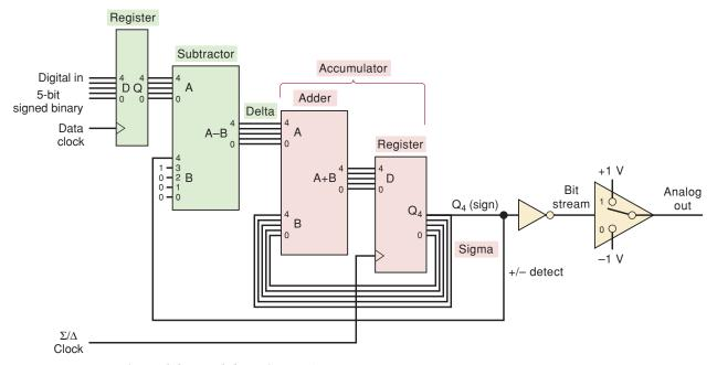
FIGURE 11-23 Sigma/delta modulator in a D/A converter.
