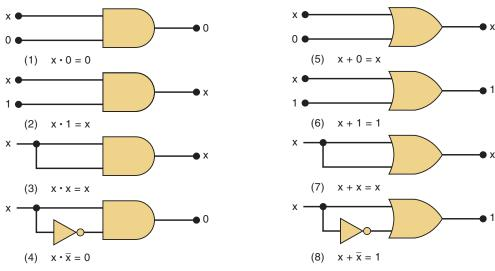
FIGURE 3-25 Single-variable theorems.
