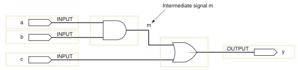
FIGURE 3-49 A logic circuit diagram with an intermediate variable.
