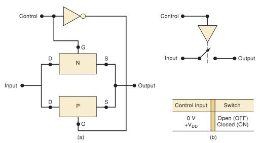
FIGURE 8-43 CMOS bilateral switch (transmission gate).
