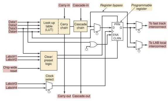
FIGURE 13-16 FLEX10K logic element. (Courtesy of Altera Corporation.)
