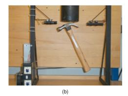
**FIGURE 1-2** A magnetic levitation system suspending: (a) a globe with a steel plate inserted and (b) a hammer.
