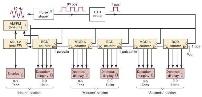
FIGURE 10-17 Block diagram for a digital clock.
