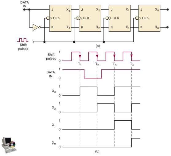
FIGURE 5-45 Four-bit shift register.
