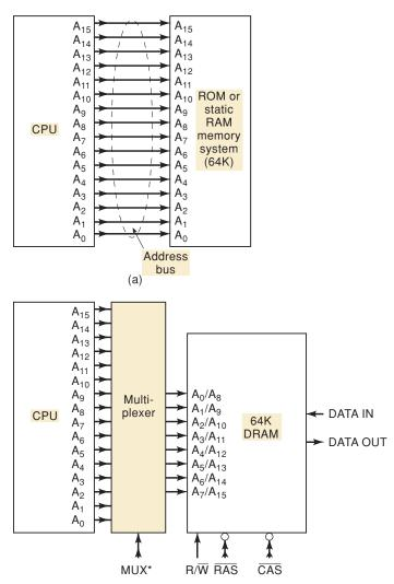
\*MUX = 0 transmits CPU address  $A_8-A_{15}$  to DRAM. MUX = 1 transmits  $A_0-A_7$  to DRAM. (b)
