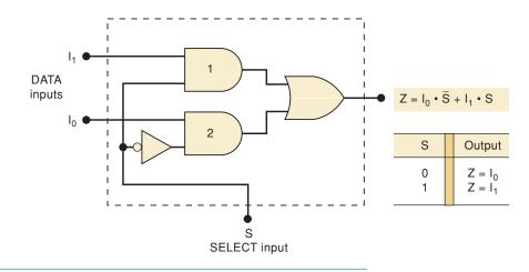
other. Using the circuit of Figure 9-19, the 10-MHz clock would be tied to  $I_0$ , and the 4.77-MHz clock would be tied to  $I_1$ . A signal from the system's control logic section would drive the SELECT input to control which clock signal appears at output Z for routing to the other parts of the circuit.
