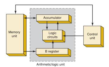
data that are stored in the memory and to execute arithmetic and logic operations on these data according to instructions from the control unit.
