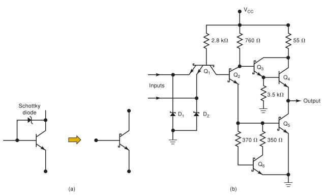
FIGURE 8-12 (a) Schottky-clamped transistor; (b) basic NAND gate in S-TTL series.
