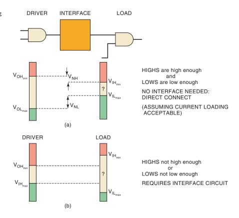
the requirements of the load. In digital systems this is pretty simple, because each device is either on or off. The interface must ensure that when the driver outputs a HIGH, the load receives a signal it perceives to be HIGH; and, when the driver outputs a LOW, the load receives a signal it perceives to be LOW.
