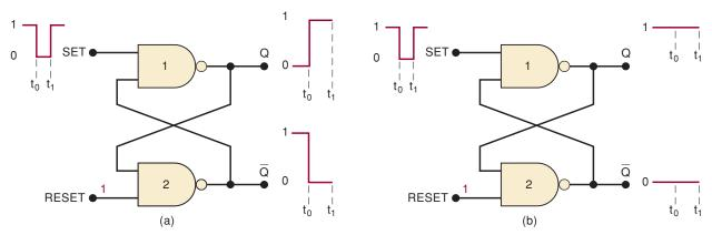
**FIGURE 5-4** Pulsing the SET input to the 0 state when (a) Q = 0 prior to SET pulse; (b) Q = 1 prior to SET pulse. Note that, in both cases, Q ends up HIGH.
