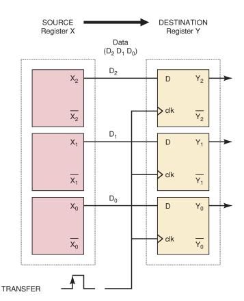
contents of the X register into the Y register is a synchronous transfer. It is also referred to as a parallel transfer because the contents of  $X_2$ ,  $X_1$ , and  $X_0$  are transferred *simultaneously* into  $Y_2$ ,  $Y_1$ , and  $Y_0$ , respectively. If a **serial data transfer** were performed, the contents of the X register would be transferred to the Y register one bit at a time. This will be examined in the next section.
