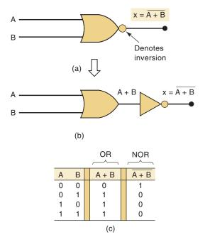
The truth table in Figure 3-19(c) shows that the NOR gate output is the exact inverse of the OR gate output for all possible input conditions. An OR gate output goes HIGH when any input is HIGH; the NOR gate output goes LOW when any input is HIGH. This same operation can be extended to NOR gates with more than two inputs.
