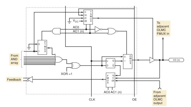
**FIGURE 13-8** Output logic macrocell for the GAL 16V8. (Reprinted with permission of Lattice Semiconductor.)
