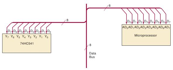
**FIGURE 9-49** Bundle method for simplified representation of data bus connections. The "/8" denotes an eight-line data bus.
