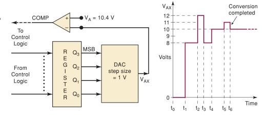
At the next step (time  $t_1$ ), the control logic sets the MSB of the register to 1 so that [Q] = 1000. This produces  $V_{AX} = 8$  V. Because  $V_{AX} < V_A$ , the COMP output is still HIGH. This HIGH tells the control logic that the setting of the MSB did not make  $V_{AX}$  exceed  $V_A$ , so that the MSB is kept at 1.
