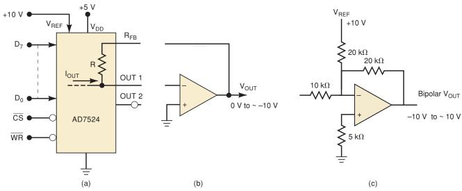
**FIGURE 11-9** (a) AD7524 8-bit DAC with latched inputs; (b) op-amp current-to-voltage converter provides 0 to approximately 10 V out; (c) op-amp circuit to produce bipolar output from -10 V to approximately +10 V.
