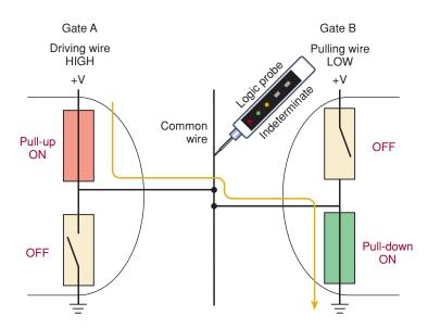
**FIGURE 8-29** Totem-pole outputs tied together can produce harmful current through  $Q_4$ .
