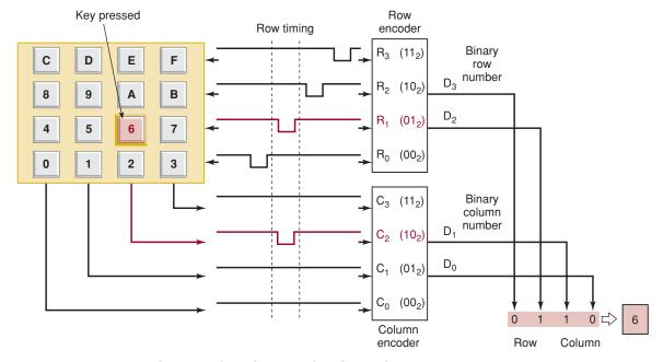
**FIGURE 10-12** Encoder operation when pressing the "6" key.
