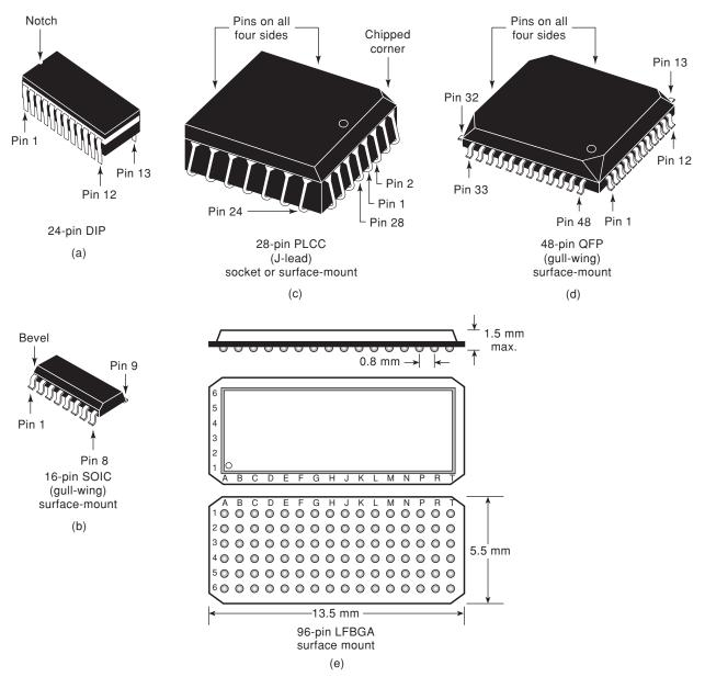
FIGURE 8-6 Common IC packages. (Courtesy of Texas Instruments)
