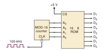
each input pulse. Assume that the ROM is programmed as in Figure 12-6, and sketch the waveforms at each ROM output as the pulses are applied. Ignore ROM delay times. Assume that the counter starts at 0000.
