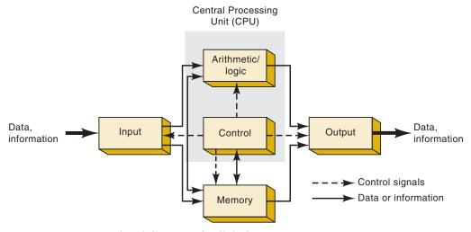
FIGURE 1-12 Functional diagram of a digital computer.
