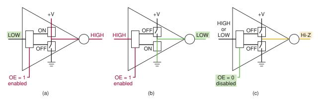
FIGURE 8-35 Three output conditions of tristate.
