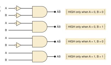
Let us now consider the case shown in Figure 4-6(a), where we have a truth table that indicates that the output x is to be 1 for two different cases: A = 0, B = 1 and A = 1, B = 0. How can this be implemented? We know that
