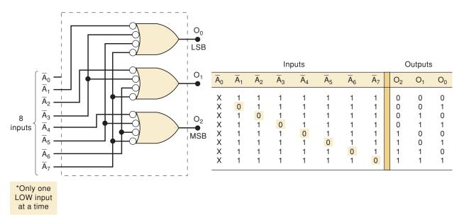
**FIGURE 9-13** Logic circuit for an octal-to-binary (8-line-to-3-line) encoder. For proper operation, only one input should be active at one time.
