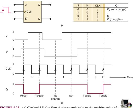
**FIGURE 5-23** (a) Clocked J-K flip-flop that responds only to the positive edge of the clock; (b) waveforms.
