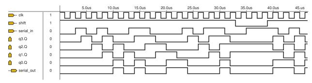
FIGURE 7-78 SISO register simulation.
