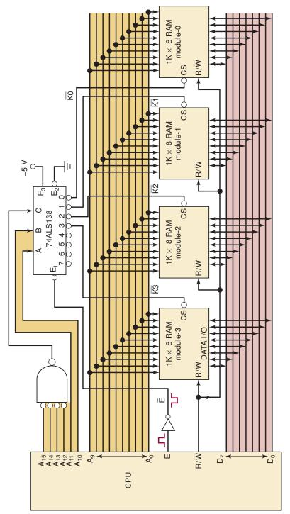
FIGURE 12-42  $4K \times 8$  RAM memory connected to a CPU.
