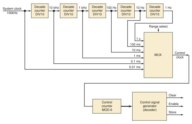
**FIGURE 10-41** Timing and control block for frequency counter.
