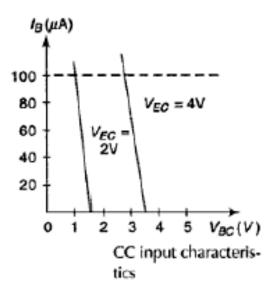
To determine input characteristics, the emitter base voltage  $V_{EB}$  is kept constant at zero and base current  $I_B$  is increased from zero by increasing  $V_{BC}$ .
