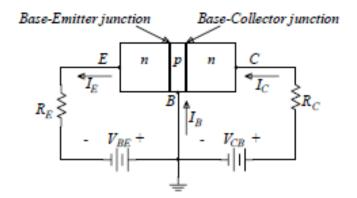
With the voltage  $V_{BE}$  and  $V_{CB}$  as shown, the Base-Emitter (B-E) junction is forward biased and the Base Collector (B-C) junction is reverse biased.
