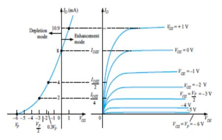
Fig 3. Drain and transfer characteristics
