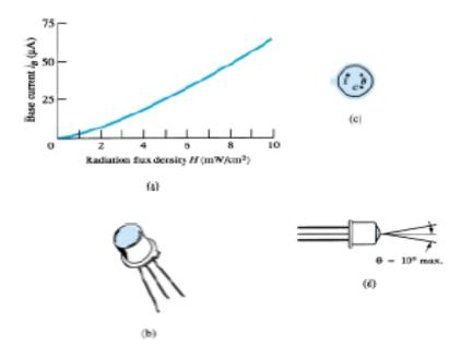
Phototransistor (a) base current vs flux density (b) Device (c) Terminal identification (d) angular alignment
