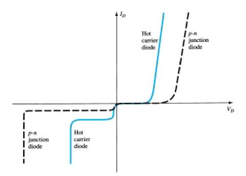
Fig 2. Comparison of characteristics of Hot carrier and pn diode
