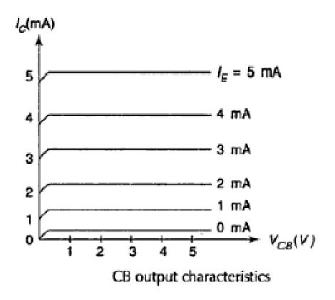
In CB configuration a variation of the base-collector voltage results in a variation of the quasineutral width in the base. The gradient of the minority-carrier density in the base therefore changes, yielding an increased collector current as the collector-base current is increased. This effect is referred to as the Early effect.
