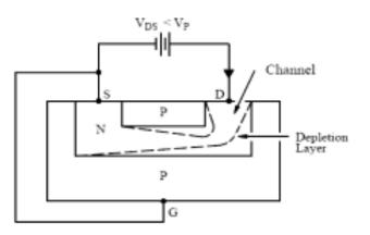
• Because the flow of current along the channel from the (+ve) drain to the (-ve) source is really a flow of free electrons from S to D in the n-type Si, the magnitude of this current will fall as more Si becomes depleted of free electrons.
