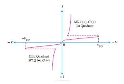
The V-I curve for triac in the Ist and IIIrd quadrants are essentially identical to SCR in the Ist quadrant.
