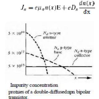
An electric field will occur in the base if non uniform doping exists in the base. Electric field can be written as
