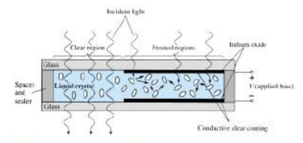
Figure 2 Nematic liquid crystal with applied bias.
