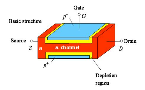
N-channel devices have greater conductivity than p-channel types, since electrons have higher mobility than do holes; thus n-channel JFETs are approximately twice as efficient conductors compared to their p-channel counterparts.
