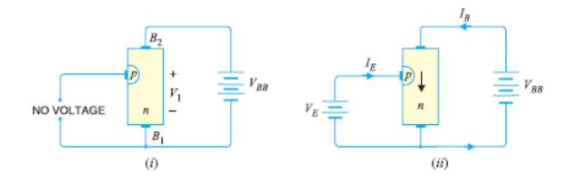
The device has normally B2 is positive w.r.t B1.
