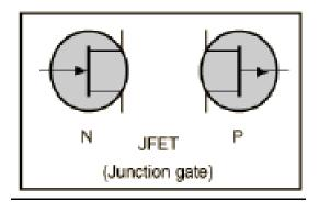
JFETs consists of a piece of high-resistivity semiconductor material (usually Si) which constitutes a channel for the majority carrier flow.
