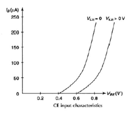
Here the base width decreases. So curve moves right as  $V_{CE}$  increases.
