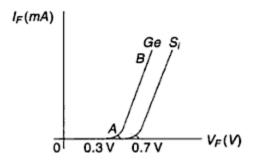
For  $V_F > Vo$ , the potential barrier at the junction completely disappears and hence, the holes cross the junction from P to N type and electrons cross the junction to opposite direction, resulting large current flow in external circuit.
