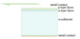
Diagram of a simple laser diode, such as shown above; not to scale
