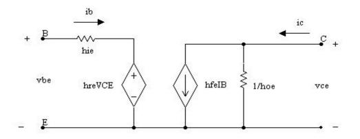
Short Circuit Input Impedance hii = ZiN with output shorted  $<\Omega>$ hu = Vi
