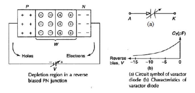
• They are also called voltage-variable capacitance diodes.
