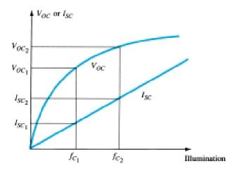
Fig 3. Voc and Isc versus illumination for solar cell
