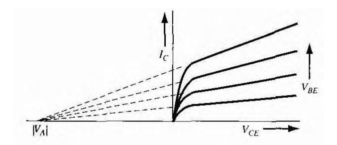
Collector current increase with an increase of the collector-emitter voltage due to the Early effect. The Early voltage,  $V_A$ , is also indicated on the figure.
