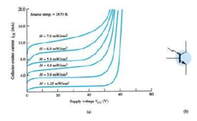
Photo Transistor (a) collector characteristics (b) symbol
