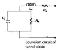
• This is the equivalent circuit of tunnel diode when biased in negative resistance region.
