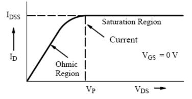
• Increasing V<sub>DS</sub> increases the widths of depletion layers, which penetrate more into channel and hence result in more channel narrowing toward the drain.
