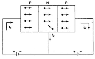
Fig. 6.5 Current in PNP transistor
