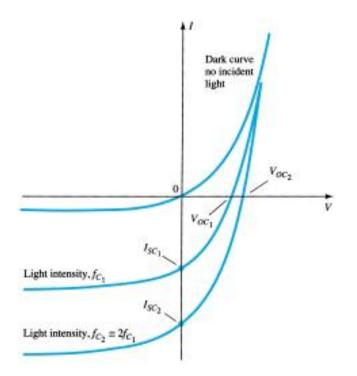
Fig 2. V-I curve for solar cell
