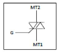
The three terminals on a triac are called Main Terminal 1 (MT1), Main Terminal 2(MT2) and Gate (G). To turn on the triac there needs to be a small current IGT flowing through the gate, this current will only flow when the voltage between G and MT1 is at least VGT. The signal that turns on the triac is called the trigger signal. Once the triac is turned on it will stay on even if there is no gate current until the current flowing between MT2 and MT1 fall below the hold current IH.
