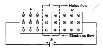
The applied potential in external battery acts in opposition to the internal potential barrier which disturbs the equilibrium.
