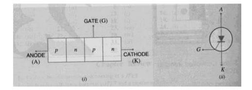
When a pn junction is added to a junction transistor the resulting three pn junction device is called a SCR. ordinary rectifier (pn) and a junction transistor (npn) combined in one unit to form
