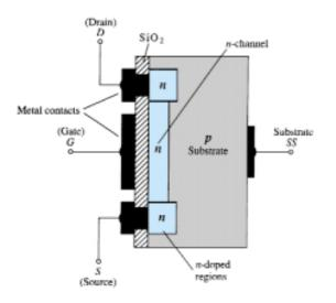
Fig. 1 n – channel depletion type MOSFET
