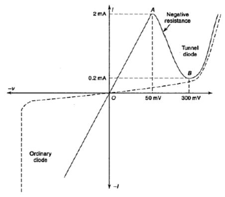
V-I characteristic of tunnel diode
