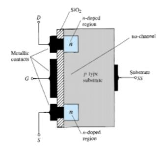
Fig 1. N channel enhancement type MOSFET
