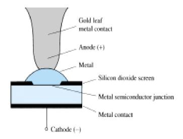
Fig 1. Passivated schottky barrier diode
