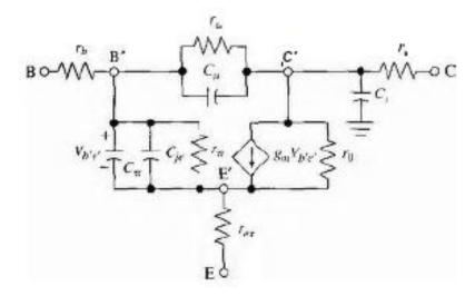
Figure 3 Hybrid-pi equivalent circuit.
