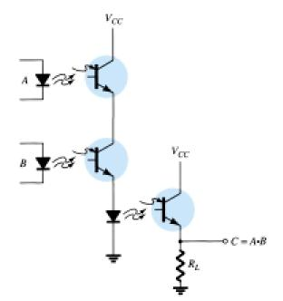
High isolation AND gate employing phototransistor and LED
