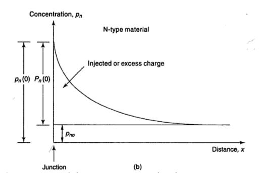
(a) Exess hole concentration varying along the axis in an N-type semiconductor bar
