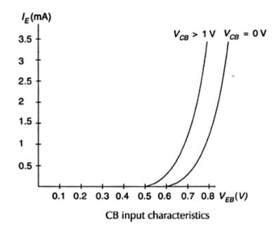
When  $V_{CB}$  is zero EB junction is forward biased. So it behaves as a diode so that emitter current increases rapidly.
