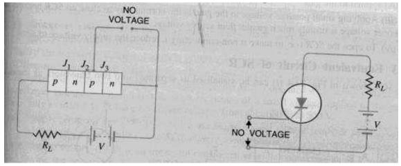
No voltage applied to the gate, j2 is reverse biased while j1 and j3 are FB. J1 and J3 is just in npn transistor with base open .no current flows through the load RL and SCR is cut off. If the applied voltage is gradually increased a stage is reached when RB junction J2 breakdown .the SCR now conducts heavily and is said to be ON state. the applied voltage at which SCR conducts heavily without gate voltage is called Break over Voltage.
