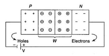
Hence, the width of the depletion region which is depleted of mobile charge carriers increases. Thus, the electric field produced by applied reverse bias, is in the same direction as the electric field of the potential barrier.
