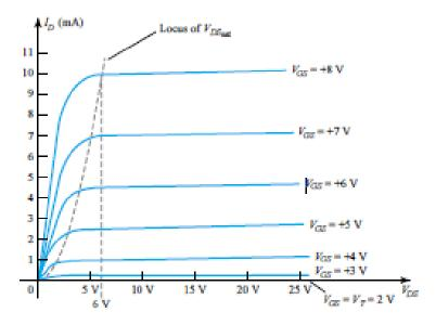
Fig 4. Drain characteristics
