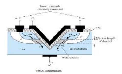
There is also the existence of two conduction paths between drain and source, as shown in Fig., to further contribute to a higher current rating. The net result is a device with drain currents that can reach the ampere levels with power levels exceeding 10 W.
