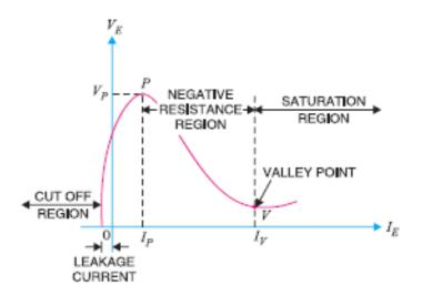
Initially in the cut off region, as  $V_E$  increases from zero, slight leakage current flows from terminalB2 to the emitter.
