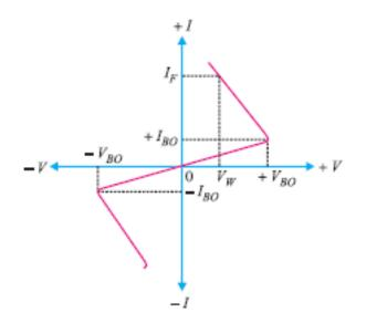
For applied positive voltage less than + Vbo and Negative voltage less than -Vbo, a small leakage current flows thrugh the device. Under such conditions the diac blocks flow of current and behaves as an open circuit. the voltage +Vbo and -Vbo are the breakdown voltages and usually have range of 30 to 50 volts.
