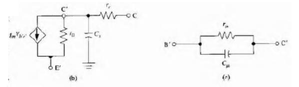
Figure 2 | Components of the hybrid-pi equivalent circuit between (a) the base and emitter, (h) the collector and emitter. and (c) the base and collector.
