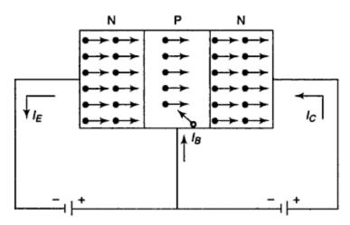
Fig. 6.4 Current in NPN transistor
