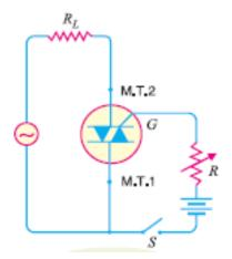
If terminal MT2 is positive w.r.t MT1 the triac is on and the conventional current will flow from MT2 to MT1.
