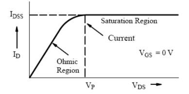
• With a steady gate-source voltage of 1 V there is always 1 V across the wall of the channel at the source end.
