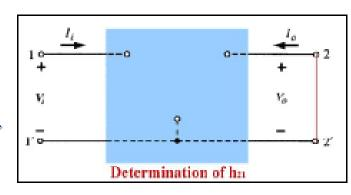
Short Circuit Forward Transfer Ratio h21 = <dimensionless>
