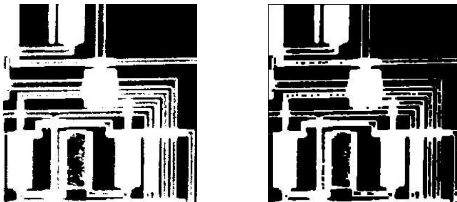
Figure 11.8: Erosion of a binary image
