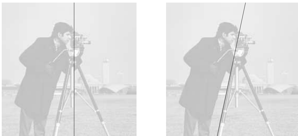
Figure 10.12: The houghline function in action
