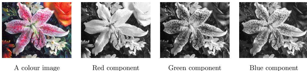
Figure 12.12: An RGB colour image and its components
