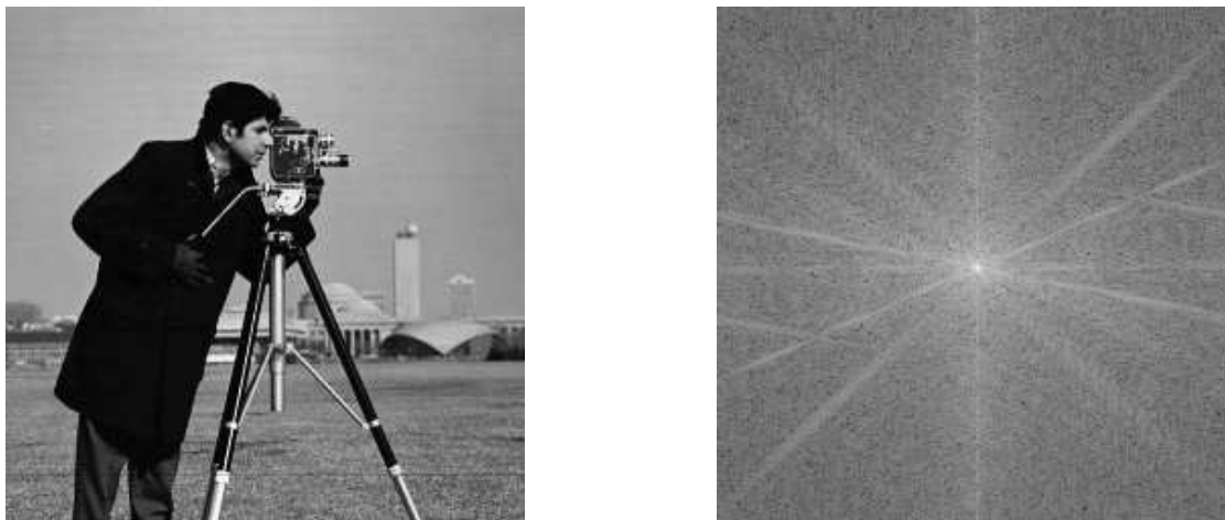
Figure 9.14: The “cameraman” image and its DFT
