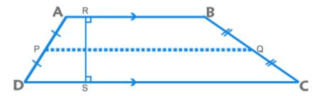
A quadrilateral with exactly one pair of sides parallel is known as a Trapezoid. The parallel sides are known as bases and the non-parallel sides are known as lateral sides.
