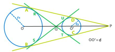
Length of the Direct Common Tangent (DCT)
