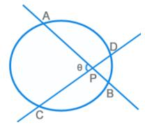
PA x PB = PC x PD  $\theta = \frac{1}{2} [m(Arc AC) + m(Arc BD)]$
