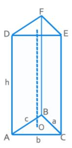
It is a solid with rectangular vertical faces and bases as congruent polygons (of n sides). It will have '2n' Vertices; 'n+2' Faces and '3n' Sides / Edges.
