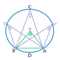
A chord /arc subtends equal angle at any point on the circumference and double of that at the centre.
