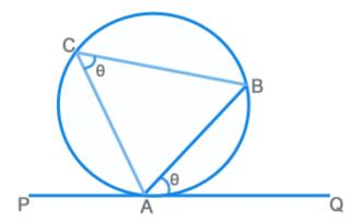
The angle made by the chord AB with the tangent at A (PQ) is equal to the angle that it subtends on the opposite side of the circumference.
