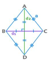
A parallelogram with all sides equal is a Rhombus. Its diagonals bisect at 90°.
