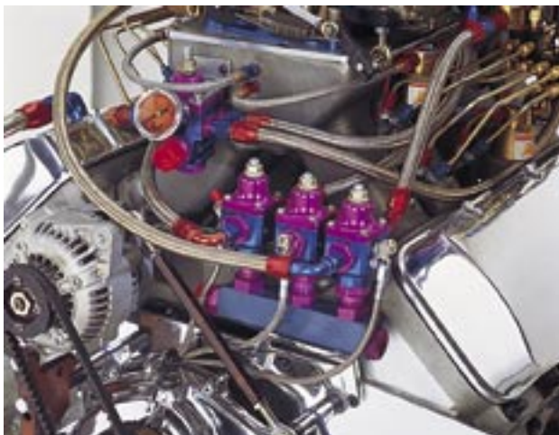
MagnaFuel's Regulators shown mounted on an engine in a nitrous-oxide configuration.
