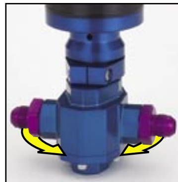
Swivel flange allows you to loosen pinch bolt and swivel the head 360° after the pump is mounted to optimize the fuel line routing.
