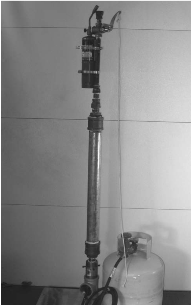
Flamethrower completed (heat-resistant cloth not shown for clarity)
