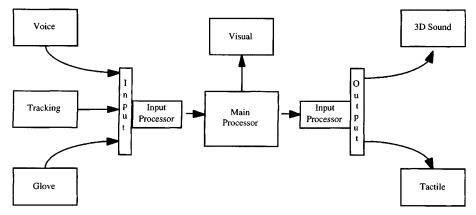
Fig. 14.2 VR system architecture.
