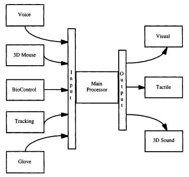
Fig. 14.1 Hardware in a VR system.
