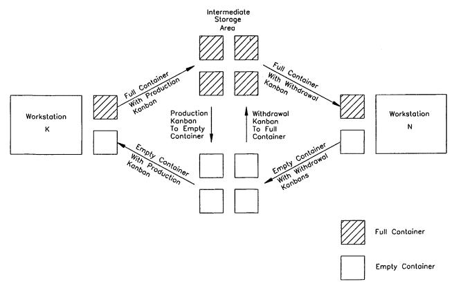
Fig. 32.16 Example of a two-card Kanban system.
