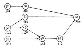
Fig. 32.15 Precedence diagram for automobile backup-light assembly. (From Ref. 39.)
