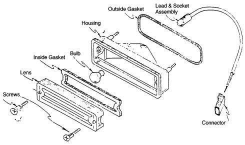
Fig. 32.14 Automobile back-up light assembly. (From Ref. 39.)
