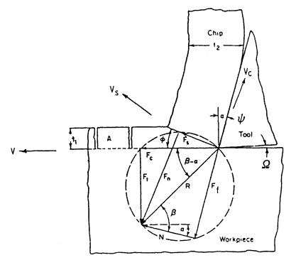
Fig. 33.2 Mechanics of metal-cutting process.
