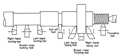
Fig. 33.9 Common lathe operations.
