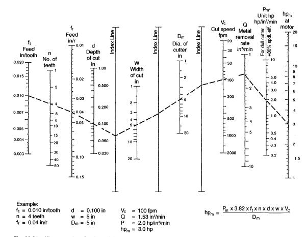
Fig. 33.21 Alignment chart for determining metal removal rate and motor horsepower in face milling-English units.
