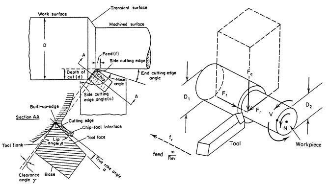
Fig. 33.10 Tool geometry-external turning.
