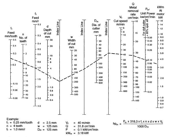
Fig. 33.22 Alignment chart for determining metal removal rate and motor power in face milling-metric units.
