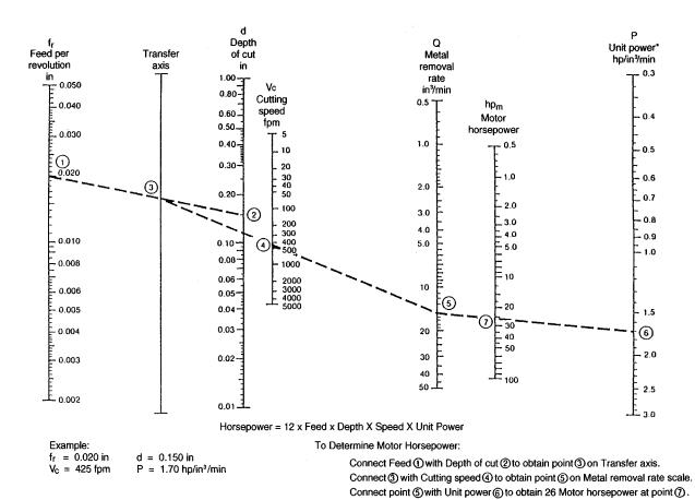
Fig. 33.11 Alignment chart for determining metal removal rate and motor horsepower in turning—English units.
