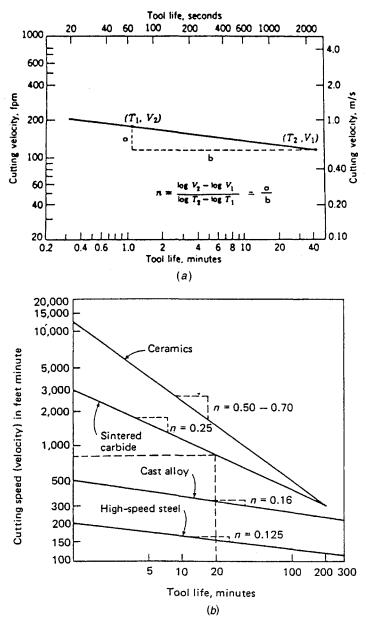
Fig. 33.6 Cutting speed/tool life relationship.
