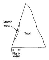
Fig. 33.5 Types of tool wear.
