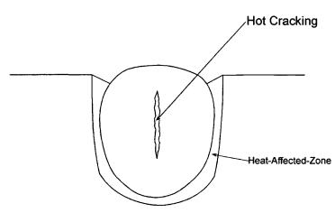
Fig. 35.32 Deeply penetrating weld made by SAW process with hot cracking.
