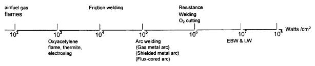
Fig. 35.30 Spectrum of practical heat intensities used for fusion welding.
