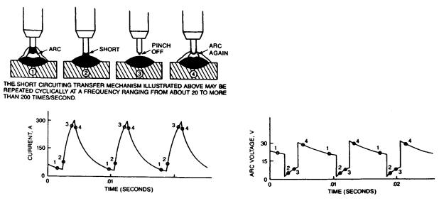
Fig. 35.35 GMAW process operating in the short-circuiting transfer mode.
