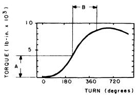
Fig. 35.28 In turn-of-nut techniques, the nut is first tightened with an approximate torque (A) and then further tightened with a measured turn (B).
