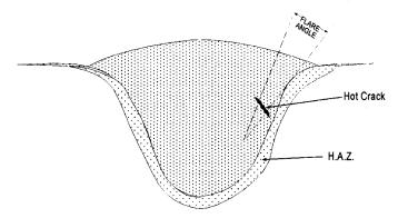
Fig. 35.33 Weld made by SAW with flare angle and hot cracking at juncture of 2 solidification fronts.
