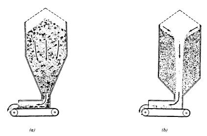
Fig. 38.7 Mass-flow (a) and funnel-flow (b) in storage bins.
