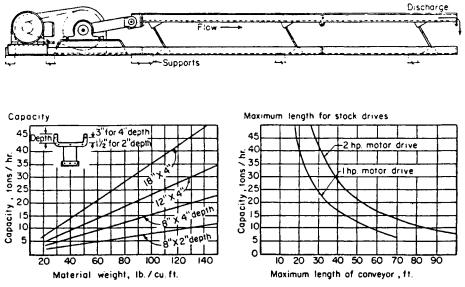
Fig. 38.4 Leaf-spring mechanical vibrating conveyor.
