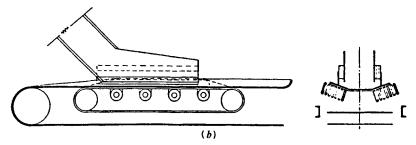
Fig. 38.2 A typical belt conveyor loading arrangement.
