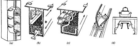
Fig. 38.5 Continuous-flow conveyor.
