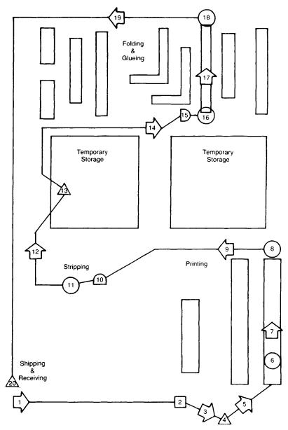
Fig. 38.16 Flow diagram.
