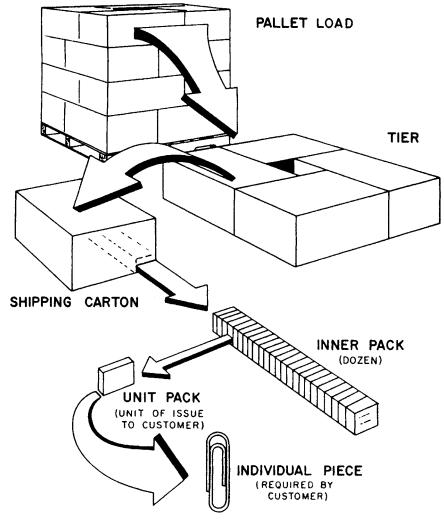
Fig. 38.19 Unit load design.
