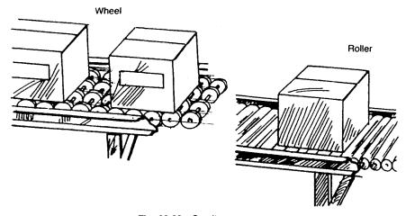
Fig. 38.23 Gravity conveyors.
