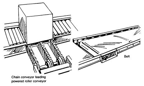
Fig. 38.24 Belt and roller conveyors.
