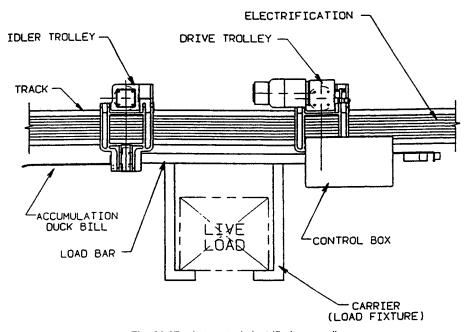
Fig. 38.27 Automated electrified monorail.
