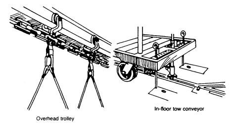
Fig. 38.25 Chain-driven conveyors.
