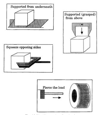
Fig. 38.22 Ways to handle a load.
