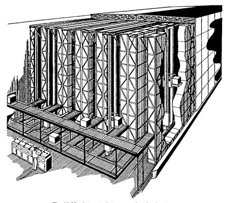
Fig. 38.32 Automated storage and retrieval system.
