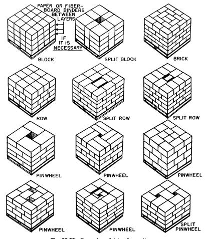
Fig. 38.20 Example pallet-loading patterns.
