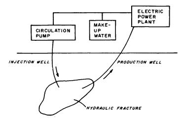
Fig. 50.2 Hot dry rock power plant configuration.
