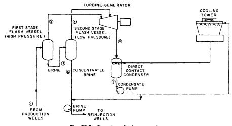
Fig. 50.6 Two-stage flash conversion.
