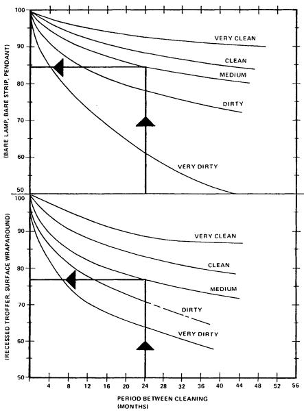
Fig. 51.1 Reduction in light output from fluorescent fixtures as a function of fixture cleaning frequency and the cleanliness of the fixture's surroundings.<sup>3</sup>
