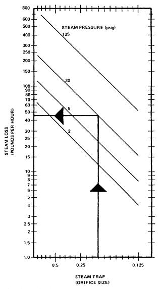
Fig. 51.2 Steam loss through leaking steam traps as a function of stem pressure and trap orifice size.<sup>3</sup>
