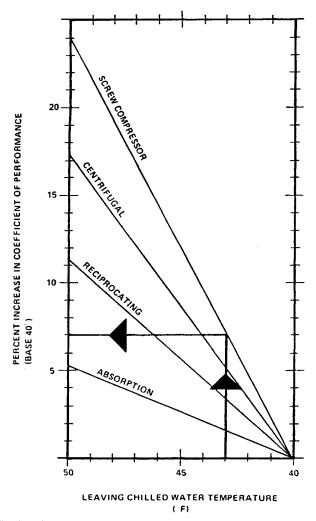
Fig. 51.4 Adjusting air-conditioner controls to provide higher chilled-water temperatures improves chiller efficiency.<sup>3</sup>
