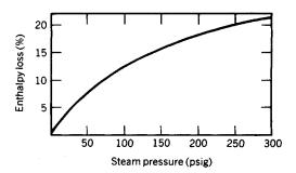
Fig. 51.3 Percentage of heat that is lost due to condensate flashing at various pressures.
