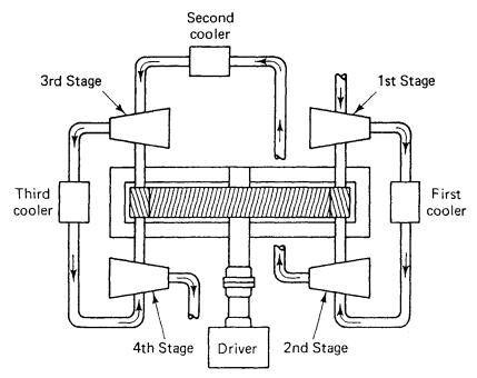
Fig. 61.7 Flow diagram of an integral-gear-type compressor showing stages of compression and including the cooling arrangement.<sup>1</sup>
