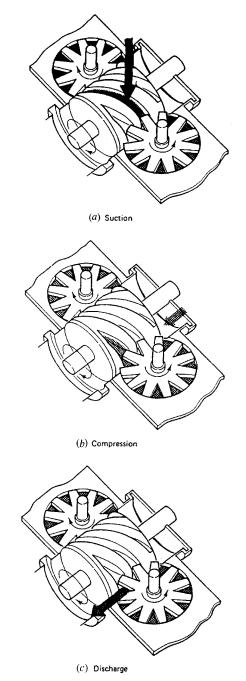
Fig. 61.4 Diagram showing the operation of the rotary, single-screw compressor.<sup>1</sup>
