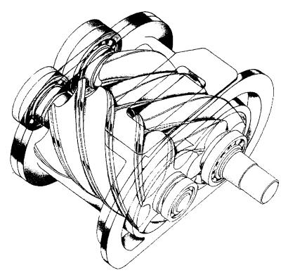
Fig. 61.5 Rotary, helical-screw compressor, typical single-stage design.<sup>1</sup>
