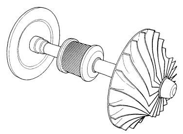
Fig. 61.6 Pinion of an intergral-gear unit having open, backward-curve-bladed impellers.<sup>1</sup>
