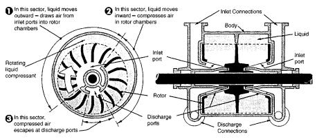
Fig. 61.10 A sectional and end view of a liquid ring compressor (courtesy of Nash Engineering Co.).<sup>2</sup>
