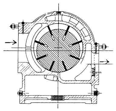
Fig. 61.8 Cross section of a sliding vane compressor (courtesy of A-C Compressor Corporation, Milwaukee, Wisconsin).<sup>2</sup>
