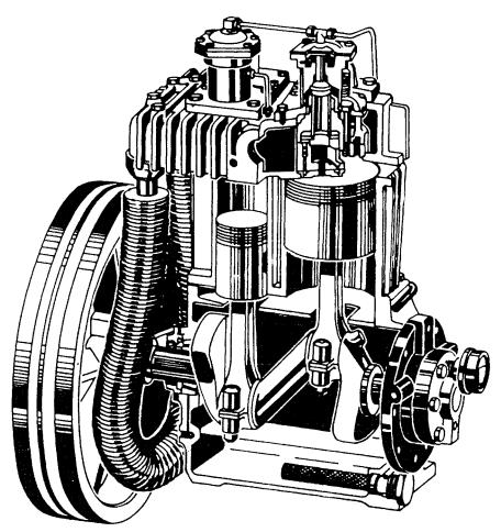
Fig. 61.2 Single-acting, two-stage compressor.1
