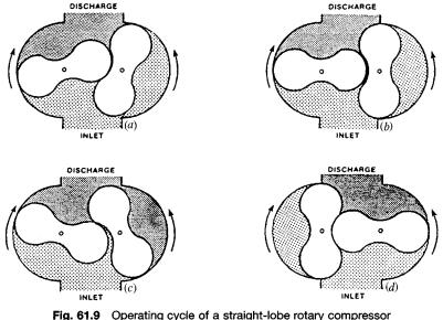
ig. 61.9 Operating cycle of a straight-lobe rotary compressor (modified; courtesy of Ingersoll-Rand).<sup>2</sup>
