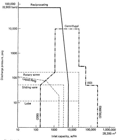
Fig. 61.1 Pressure-capacity chart showing the effective ranges of most compressors.<sup>1</sup>
