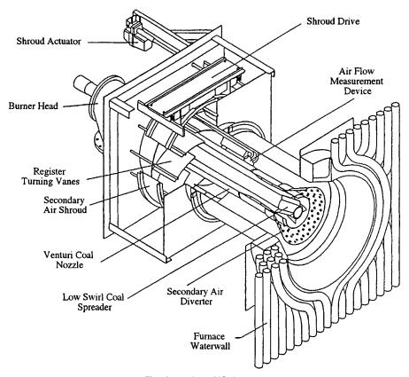
Fig. 65.1 Low-NO<sub>x</sub> burner.
