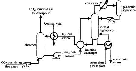
Fig. 65.3 Schematic of CO<sub>2</sub> scrubbing system.
