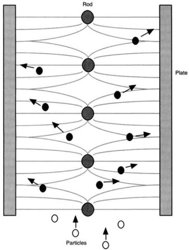
Fig. 65.2 Schematic of electrostatic precipitator operation.
