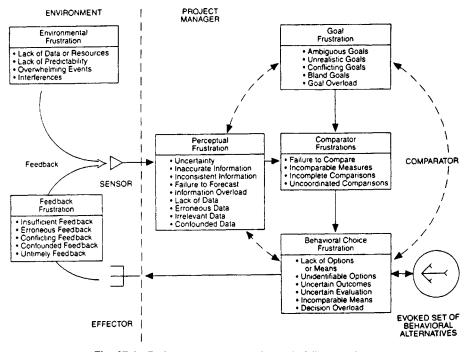
**Fig. 67.4** Project management cybernetic failure modes.
