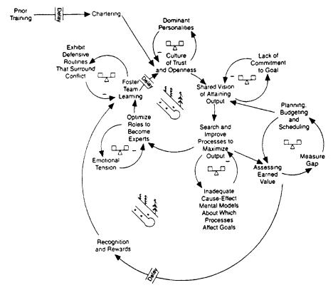
Fig. 67.10 Dynamics of a project control system.
