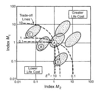
**Fig. 9.9** The proper comparison of A with competing materials is made by constructing a value-function,  $\tilde{V}$ , which combines the cost of material with that associated with weight, using the weight–cost exchange constant  $E^{\$}$ . When  $E^{\$} = 10$  /kg, C is a better choice than A; when  $E^{\$} = 0.1$  /kg, D is better than A.
