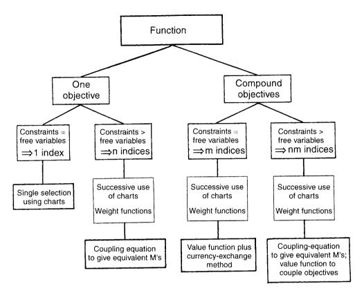
Fig. 9.1 The procedures for dealing with multiple constraints and compound objectives.
