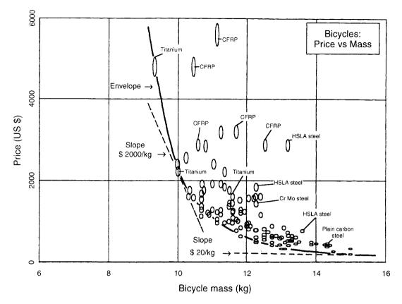
**Fig. 9.7** A plot of cost against mass for bicycles. The lower envelope of price is here treated as a contour of constant value. The exchange constant is the slope of a tangent to this curve. It varies with mass.
