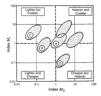
**Fig. 9.8** A schematic chart showing two indices,  $M_1^*$  measuring cost and  $M_2^*$  measuring weight. If the currently used material is A, then B is both cheaper and lighter. The material C is lighter but costs more; D is cheaper but heavier. This selection ignores the trade-off between weight and cost.
