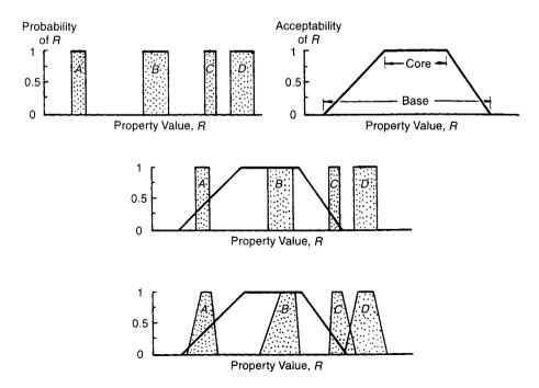
**Fig. 9.3** Fuzzy selection methods. Sharply-defined properties and a fuzzy selection criterion, shown at (a), are combined to give weight-factors for each material at (b). The properties themselves can be given fuzzy ranges, as shown at (c).
