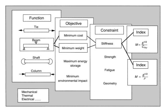
Fig. 9.6 Two objectives (here, minimizing mass and cost) and one constraint (stiffness) lead to two indices.
