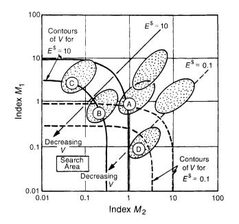
**Fig. 9.10** Selection to minimize total life-cost, using the exchange constant method. The contours show the value-function,  $\tilde{V}$ , for two values of  $E^{\$}$ .
