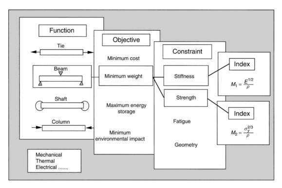
Fig. 9.2 One objective (here, minimizing mass) and two constraints (stiffness and strength) lead to two indices.
