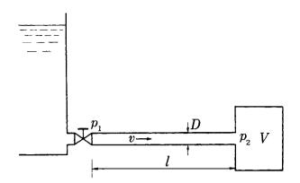
Fig. 14.3 System comprising pipe line and tank
