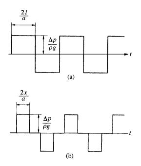
Fig. 14.7 Change in pressure due to water hammer, (a) at point C and (b) at point B in Fig. 14.6
