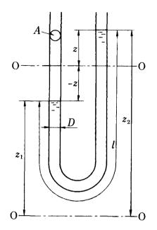
Fig. 14.1 Vibration of liquid column in a U-tube
