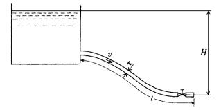
Fig. 14.4 Transient flow in a pipe
