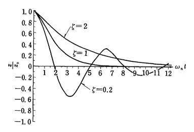
Fig. 14.2 Motion of liquid column with frictional resistance
