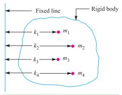
Fig. 1.4. Mass moment of inertia.
