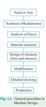
**7.** *Detailed drawing.* Draw the detailed drawing of each component and the assembly of the machine with complete specification for the manufacturing processes suggested.
