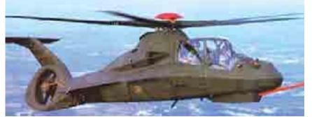
This picture shows a reconnoissance helicopter of air force. Its dark complexion absorbs light that falls on its surface. The flat and sharp edges deflect radar waves and they do not return back to the radar. These factors make it difficult to detect the helicopter.
