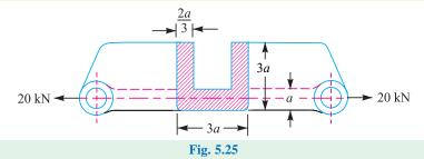
Solution. Given :  $P = 20 \text{ kN} = 20 \times 10^3 \text{ N}$  ;  $\sigma_{t(max)} = 25 \text{ MPa} = 25 \text{ N/mm}^2$  ;  $\sigma_{c(max)} = 80 \text{ MPa}$ = 80 N/mm<sup>2</sup>
