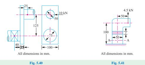
A steel bracket is subjected to a load of 4.5 kN, as shown in Fig. 5.41. Determine the required thickness of the section at A-A in order to limit the tensile stress to 70 MPa. [Ans. 9 mm]
