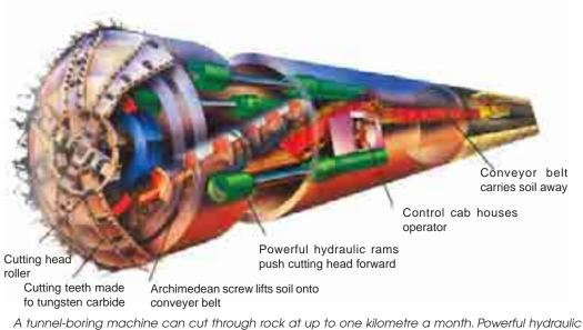
rams force the machine's cutting head fowards as the rock is cut away.
