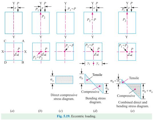
Consider a short prismatic bar subjected to a compressive load P acting at an eccentricity of e as shown in Fig. 5.19 (a).
