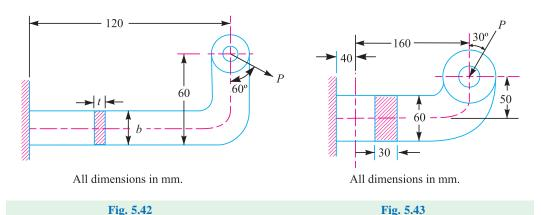
18. A bracket, as shown in Fig. 5.43, is bolted to the framework of a machine which carries a load P. The cross-section at 40 mm from the fixed end is rectangular with dimensions, 60 mm  $\times$  30 mm. If the maximum stress is limited to 70 MPa, find the value of P.
