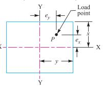
Fig. 5.20. Eccentric load with eccentricity about two axes.
