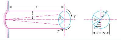
Fig. 5.1. Torsional shear stress.
