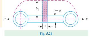
When the link is in the position shown by full lines in Fig. 5.24, the area of cross-section,
