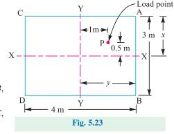
$\sigma_{A} = \frac{P}{A} + \frac{P \cdot e_{x} \cdot x}{I_{YY}} + \frac{P \cdot e_{y} \cdot y}{I_{YY}} \qquad \dots [\because At A, both x and y are +ve]$
