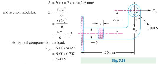
.: Bending moment due to horizontal component of the load,
