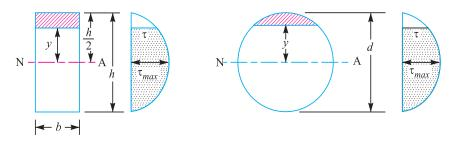
**Fig. 5.30.** Shear stress in a rectangular beam. **Fig. 5.31.** Shear stress in a circular beam.
