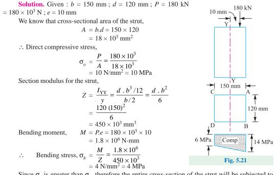
Since  $\sigma_o$  is greater than  $\sigma_b$ , therefore the entire cross-section of the strut will be subjected to compressive stress. The maximum intensity of compressive stress will be at the edge *AB* and minimum at the edge *CD*.
