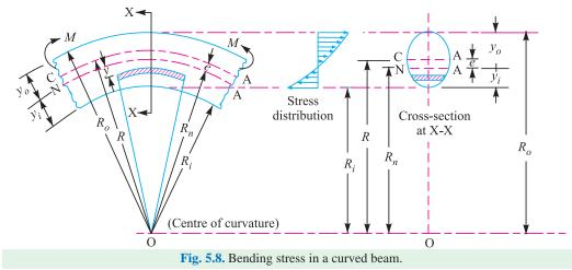
Consider a curved beam subjected to a bending moment M, as shown in Fig. 5.8. In finding the bending stress in curved beams, the same assumptions are used as for straight beams. The general expression for the bending stress ( $\sigma_{\rm b}$ ) in a curved beam at any fibre at a distance y from the neutral
