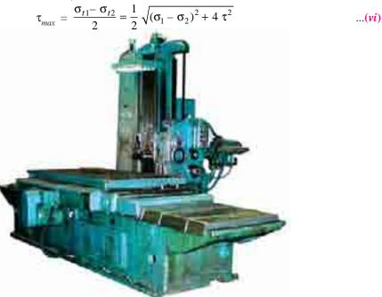
A Boring mill. Note : This picture is given as additional information and is not a direct example of the current chapter.
