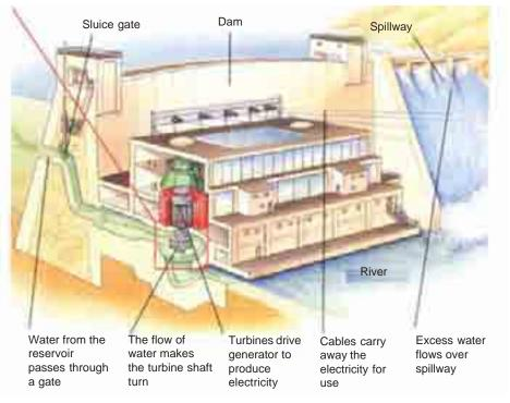
General layout of a hydroelectric plant.
