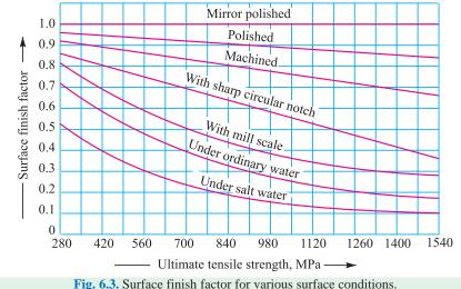
When the surface finish factor is known, then the endurance limit for the material of the machine member may be obtained by multiplying the endurance limit and the surface finish factor. We see that
