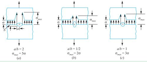
Fig. 6.6. Stress concentration due to holes.
