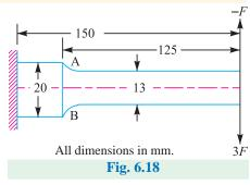
**Solution.** Given :  $W_{min} = -F$ ;  $W_{max} = 3F$ ; F.S. = 2;  $K_t = 1.42$ ; q = 0.9;  $\sigma_u = 550$  MPa = 550 N/mm<sup>2</sup>;  $\sigma_y = 470$  MPa = 470 N/mm<sup>2</sup>;  $\sigma_e = 275$  MPa = 275 N/mm<sup>2</sup>;  $K_{sz} = 0.85$ ;  $K_{sur} = 0.89$
