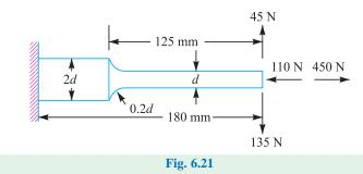
The stress concentration factors for bending and axial loads are 1.44 and 1.63 respectively, at the change of cross-section. Take size factor = 0.85 and surface finish factor = 0.9. [Ans. 12.5 mm]
