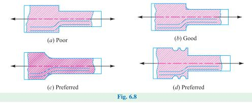
In Fig. 6.8 (*a*) we see that stress lines tend to bunch up and cut very close to the sharp re-entrant corner. In order to improve the situation, fillets may be provided, as shown in Fig. 6.8 (*b*) and (*c*) to give more equally spaced flow lines.
