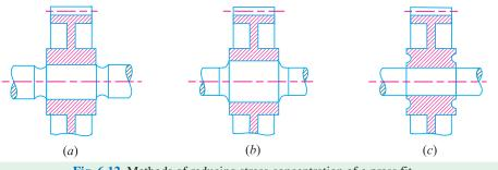
Fig. 6.12. Methods of reducing stress concentration of a press fit.
