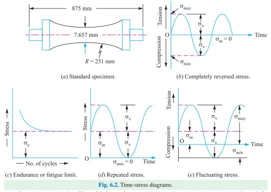
In order to study the effect of fatigue of a material, a rotating mirror beam method is used. In this method, a standard mirror polished specimen, as shown in Fig. 6.2 (*a*), is rotated in a fatigue
