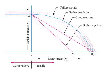
Fig. 6.15. Combined mean and variable stress.
