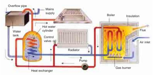
In this central heating system, a furnace burns fuel to heat water in a boiler. A pump forces the hot water through pipes that connect to radiators in each room. Water from the boiler also heats the hot water cylinder. Cooled water returns to the boiler.
