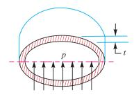
Fig. 7.5. Thin spherical shell.
