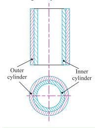
Fig. 7.8. Compound cylindrical shell.
