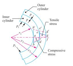
(*d*) Tangential stress distribution due to shrinkage fitting and internal fluid pressure.
