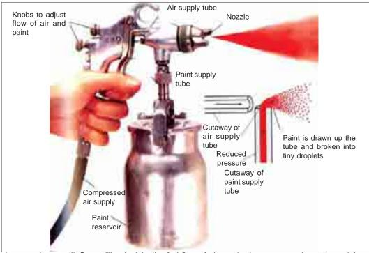
In accordance with Bernoulli's principle, the fast flow of air creates low pressure above the paint tube, sucking paint upwards into the air steam.
