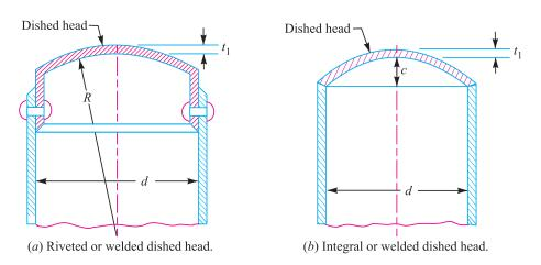
Fig. 7.12. Dished plate with uniformly distributed load.
