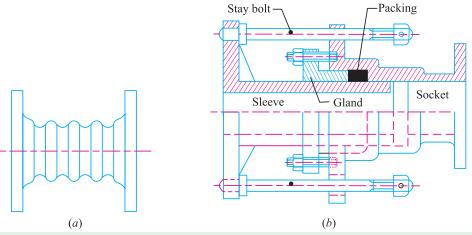
Fig. 8.7. Expansion joints.
