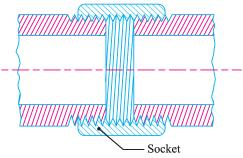
Fig. 8.2. Socket or coupler joint.
