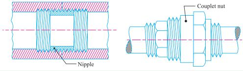
Fig. 8.3. Nipple joint.
