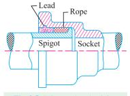
Fig. 8.5. Spigot and socket joint.
