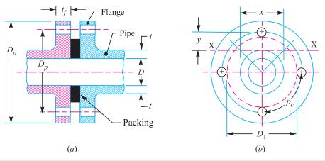
Fig. 8.8. Flanged joint.
