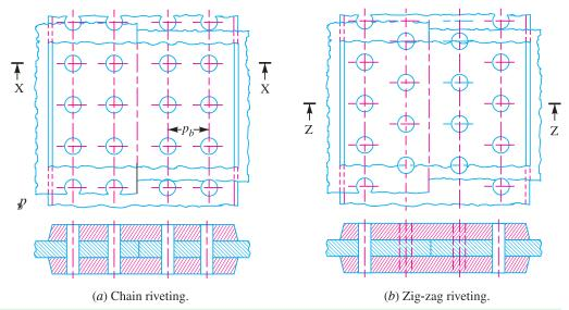
Fig. 9.9. Double riveted double strap (equal) butt joints.
