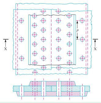
Fig. 9.11. Triple riveted double strap (unequal) butt joint.
