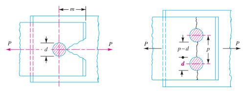
Fig. 9.13. Tearing of the plate at an edge.
