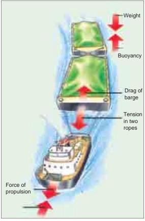
Forces on a ship as shown above need to be consider while designing various joints
