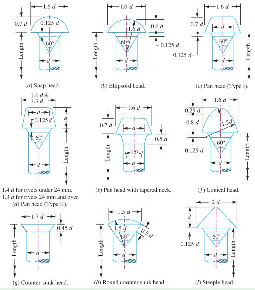
Fig. 9.5. Rivet heads for boiler work.
