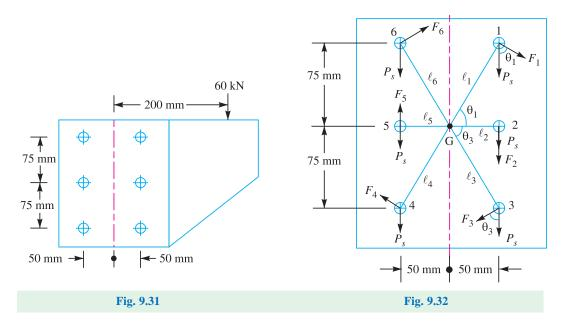
**Solution.** Given: n = 6; P = 60 kN =  $60 \times 10^3$  N; e = 200 mm;  $\tau = 150$  MPa = 150 N/mm<sup>2</sup> Since the rivets are of equal size and placed symmetrically, therefore the centre of gravity of the rivet system lies at G as shown in Fig. 9.32. We know that ditect shear load on each rivet,
