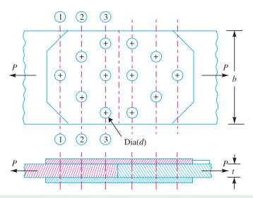
Fig. 9.19. Riveted joint for structural use.
