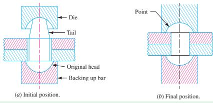
Fig. 9.2. Methods of riveting.
