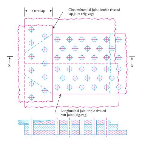
Fig. 9.18. Longitudinal and circumferential joint.
