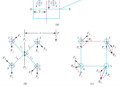
Fig. 9.23. Eccentric loaded riveted joint.
