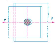
Fig. 9.17. Crushing of a rivet.
