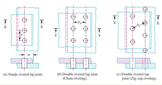
Fig. 9.6. Single and double riveted lap joints.
