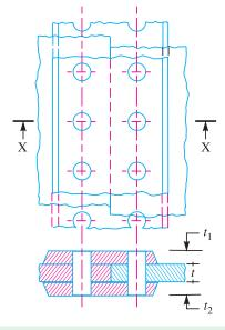
Fig. 9.8. Single riveted double strap butt joint.
