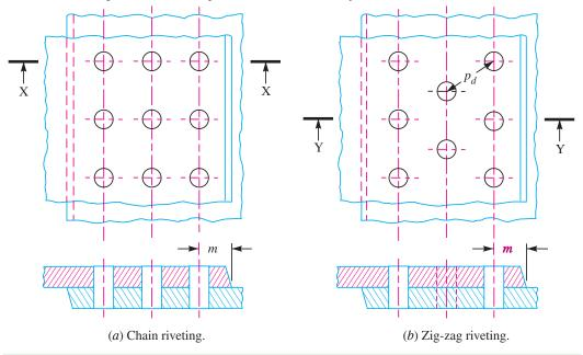
Fig. 9.7. Triple riveted lap joint.
