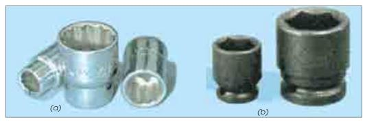
(a) Hand operated square drive sockets (b) Machine operated sockets. Note : This picture is given as additional information and is not a direct example of the current chapter.
