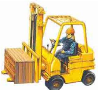
Fork lift is used to move goods from one place to the other within the factory.
