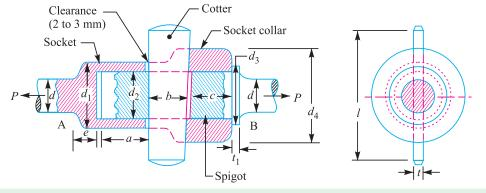
Fig. 12.1. Socket and spigot cotter joint.
