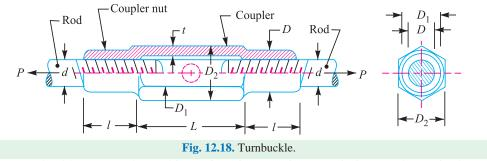
A turnbuckle commonly used in engineering practice (mostly in aeroplanes) is shown in Fig. 12.19. This type of turnbuckle is made hollow in the middle to reduce its weight. In this case, the two ends of the rods may also be seen. It is not necessary that the material of the rods and the turnbuckle may be same or different. It depends upon the pull acting on the joint.
