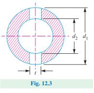
From this equation, outside diameter of socket  $(d_1)$  may be determined.
