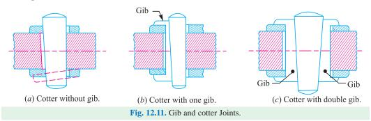
**Notes : 1.** When one gib is used, the cotter with one side tapered is provided and the gib is always on the outside as shown in Fig. 12.11 (*b*).
