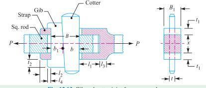
Fig. 12.13. Gib and cotter joint for square rods.
