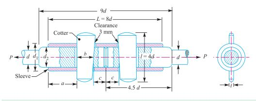
Fig. 12.9. Sleeve and cotter joint.
