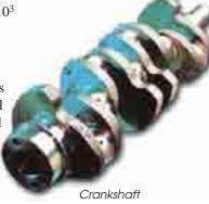
subjected to combined bending and torsion, the equivalent twisting moment,
