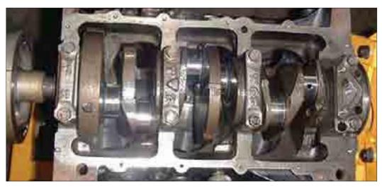
Crankshaft inside the crank-case
