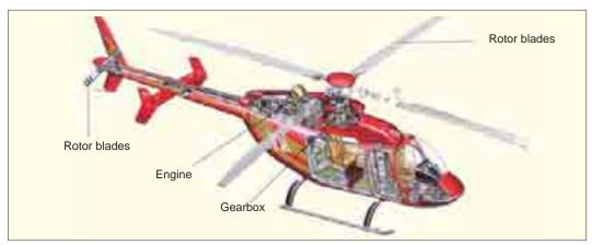
Air acclerating downwards, pushed by the rotating blades, produced an upwards reaction that lifts the helicopter.
