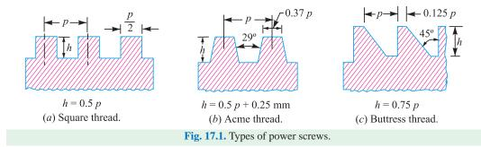
pressure on the nut. It is difficult to cut with taps and dies. It is usually cut on a lathe with a single
