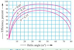
Fig. 17.5. Graph between efficiency and helix angle.
