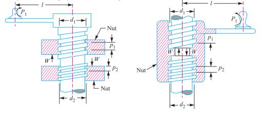
(*a*) Threads wound on the same cylinder. (*b*) Threads wound on the different cylinders. **Fig. 17.14**
