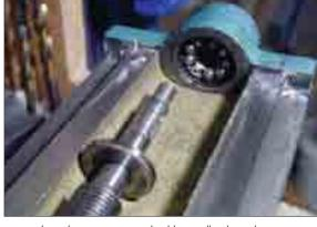
Lead screw supported by collar bearing.
