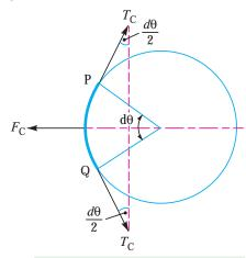
Fig. 18.18. Centrifugal tension.
