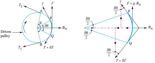
Fig. 18.16. Ratio of driving tensions for flat belt.
