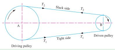
Fig. 18.15. Power transmitted by a belt.
