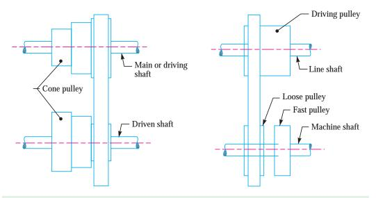
Fig. 18.10. Stepped or cone pulley drive.
