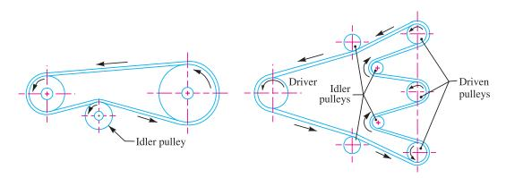
Fig. 18.7. Belt drive with single idler pulley. Fig. 18.8. Belt drive with many idler pulleys.
