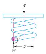
(a) Axially loaded helical spring.
