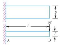
Fig. 23.25. Flat spring (cantilever type).
