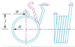
Fig. 23.23. Helical torsion spring.
