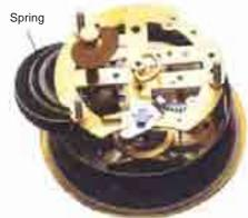
Flat spiral spring of a mechanical clock.
