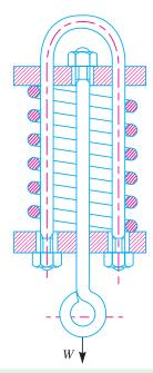
**Fig. 23.9.** Compression spring for carrying tensile load.
