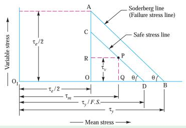
Fig. 23.19. Modified Soderberg method for helical springs.
