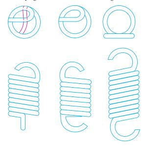
**Fig. 23.8.** End connection for tension helical springs.
