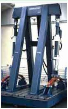
Leaf spring fatigue testing system.
