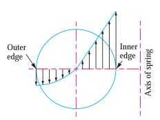
(c) Resultant torsional shear and direct shear stress diagram.
