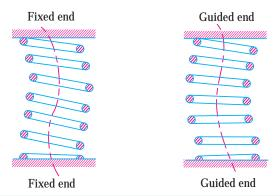
Fig. 23.13. Buckling of compression springs.
