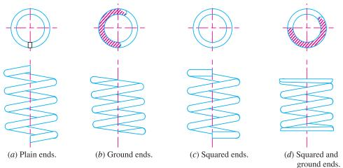
Fig 23.7. End connections for compression helical spring.
