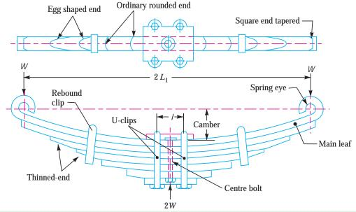
Fig. 23.30. Semi-elliptical leaf spring.
