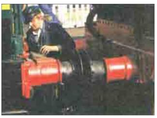
Buffers have springs inside to absorb shock.
