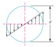
(a) Torsional shear stress diagram.
