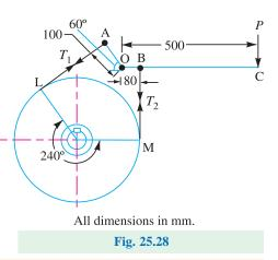
Design the steel band, shaft, key, lever and fulcrum pin. The permissible stresses may be taken as 70 MPa in tension, 50 MPa in shear and 20 MPa
