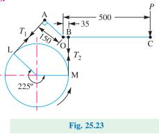
Since the length OB is greater than OA, therefore the force at the end of the lever (P) must act in the upward direction. When the drum rotates anticlockwise, the end of the band attached to A will be tight with tension  $T_1$  and the end of the band attached to B will be slack with tension  $T_2$ . First of all, let us find the values of tensions  $T_1$  and  $T_2$ . We know that
