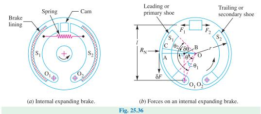
We shall now consider the forces acting on such a brake, when the drum rotates in the anticlockwise direction as shown in Fig. 25.36 (*b*). It may be noted that for the anticlockwise direction, the left hand shoe is known as *leading* or *primary shoe* while the right hand shoe is known as *trailing* or *secondary shoe*.
