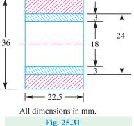
Let us now check the induced bending stress in the lever at the fulcrum. The section of the lever at the fulcrum is shown in Fig. 25.31. We know that maximum bending moment at the fulcrum,
