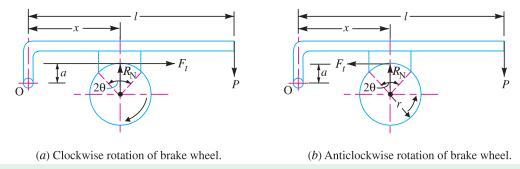
Fig. 25.3. Single block brake. Line of action of  $F_t$  passes above the fulcrum.
