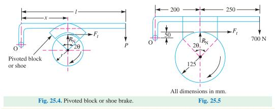
**Example 25.2.** A single block brake is shown in Fig. 25.5. The diameter of the drum is 250 mm and the angle of contact is 90°. If the operating force of 700 N is applied at the end of a lever and the coefficient of friction between the drum and the lining is 0.35, determine the torque that may be transmitted by the block brake.
