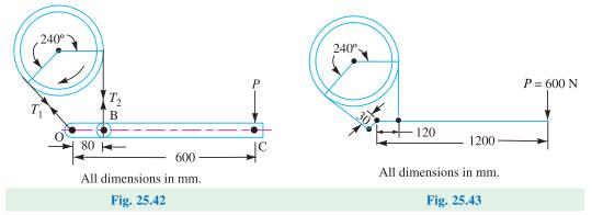
is applied at the free end of the lever, find for the clockwise and anticlockwise rotation of the drum: 1. the maximum and minimum forces in the band; and 2. the torque which can be applied by the brake.
