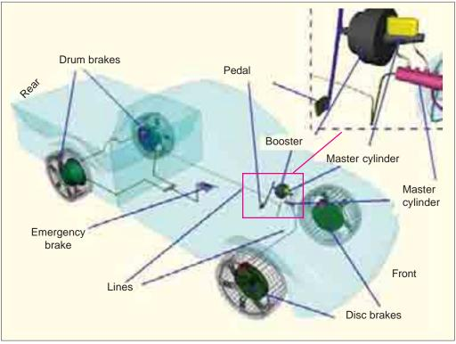
Brake System Components Note : This picture is given as additional information and is not a direct example of the current chapter.
