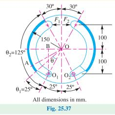
**Solution.** Given : b = 35 mm;  $\mu = 0.4$ ; r = 150 mm; l = 200 mm;  $\theta_1 = 25^\circ$ ;  $\theta_2 = 125^\circ$
