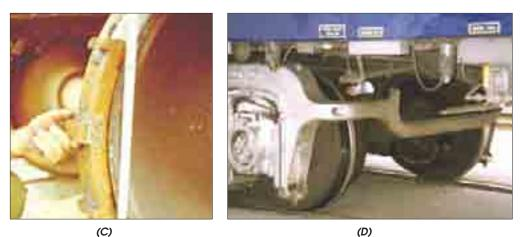
Train braking system : (C) Shoe of the train brake (D) Overview of train brake
