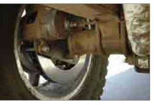
Inside view of a truck disk brake
