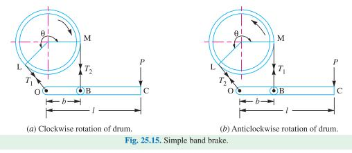
3. If the permissible tensile stress ( $\sigma_t$ ) for the material of the band is known, then maximum tension in the band is given by
