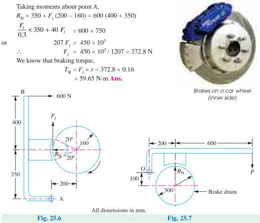
**Example 25.4.** The block brake, as shown in Fig. 25.7, provides a braking torque of 360 N-m. The diameter of the brake drum is 300 mm. The coefficient of friction is 0.3. Find :
