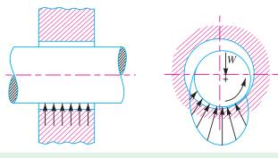
Fig. 26.5. Variation of pressure in the converging film.
