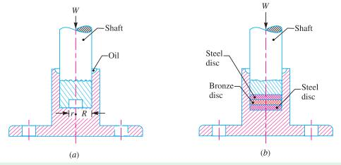
Fig. 26.14. Footstep or pivot bearings.
