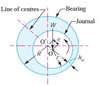
**Note :** The diametral clearance (c) in a bearing should be small **Fig. 26.7.** Hydrodynamic journal bearing. enough to produce the necessary velocity gradient, so that the pressure built up will support the load. Also the small clearance has the advantage of decreasing side leakage. However, the allowance must be made for manufacturing tolerances in the journal and bushing. A commonly used clearance in industrial machines is 0.025 mm per cm of journal diameter.
