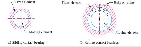
Fig. 26.2. Sliding and rolling contact bearings.
