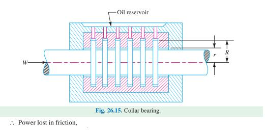
$$P = \frac{2\pi N.T}{60} \text{ watts} \qquad \dots \text{ (when } T \text{ is in N-m)}$$
