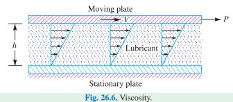
When the thickness of the fluid lubricant is small which is the case for bearings, then the velocity gradient is very nearly constant as shown in Fig. 26.6, so that
