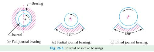
The sliding contact bearings in which the sliding action is along the circumference of a circle or an arc of a circle and carrying radial loads are known as *journal* or *sleeve bearings*. When the angle of contact of the bearing with the journal is 360° as shown in Fig. 26.3 (*a*), then the bearing is called a *full journal bearing*. This type of bearing is commonly used in industrial machinery to accommodate bearing loads in any radial direction.
