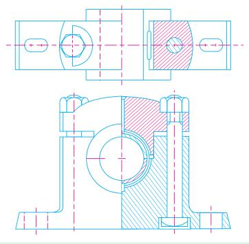
Fig. 26.11. Split bearing or plummer block.
