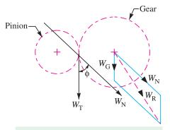
Fig. 28.16. Load acting on the gear.
