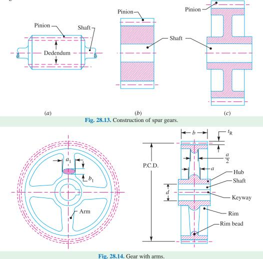
Large gears are provided with arms to join the hub and the rim, as shown in Fig. 28.14. The number of arms depends upon the pitch circle diameter of the gear. The number of arms may be selected from the following table.
