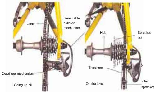
Bicycle gear mechanism switches the chain between different sized sprockets at the pedals and on the back wheel. Going up hill, a small front and a large rear sprocket are selected to reduce the push required for the rider. On the level, a large front and small rear, sprocket are used to prevent the rider having to pedal too fast.
