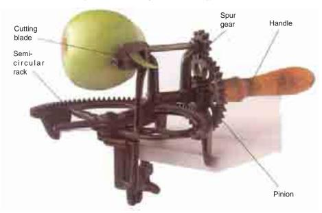
**Kitchen Gear**: This 1863 fruit and vegetable peeling machine uses a rack and pinion to drive spur gears that turn an apple against a cutting blade. As the handle is pushed round the semi-circular base, the peel is removed from the apple in a single sweep.
