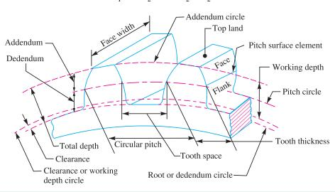
Fig. 28.6. Terms used in gears.
