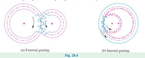
In *external gearing*, the gears of the two shafts mesh externally with each other as shown in Fig. 28.4 (a). The larger of these two wheels is called *spur wheel* or *gear* and the smaller wheel is called *pinion*. In an external gearing, the motion of the two wheels is always unlike, as shown in
