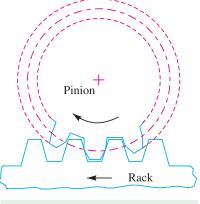
Fig. 28.5. Rack and pinion.
