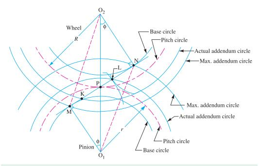
Fig. 28.11. Interference in involute gears.
