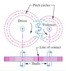
Fig. 28.1. Friction wheels.
