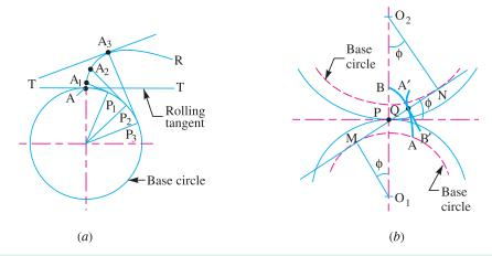
Fig. 28.10. Construction of involute teeth.
