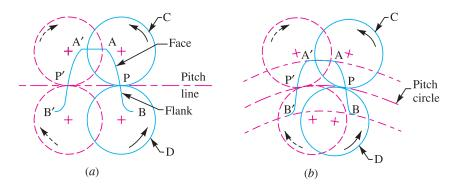
Fig. 28.8. Construction of cycloidal teeth of a gear.
