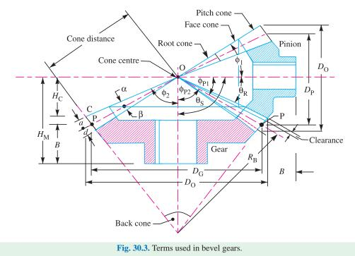
A sectional view of two bevel gears in mesh is shown in Fig. 30.3. The following terms in connection with bevel gears are important from the subject point of view :
