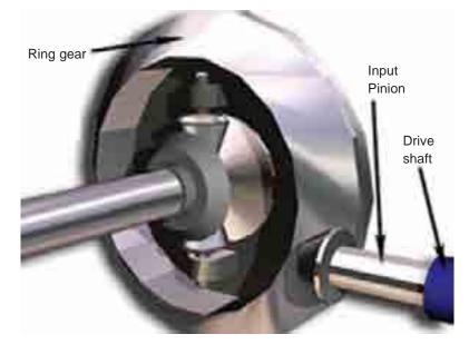
Hypoid bevel gears in a car differential
