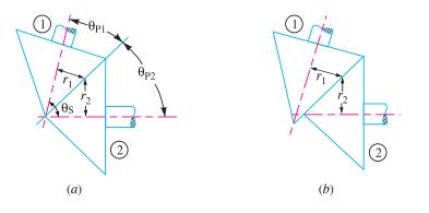
Fig. 30.1. Pitch surface for bevel gears.
