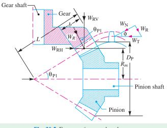
Fig. 30.5. Forces acting on a bevel gear.
