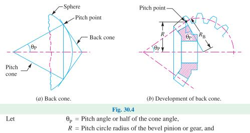
$R_{\rm B}$  = Back cone distance or equivalent pitch circle radius of spur pinion or gear.
