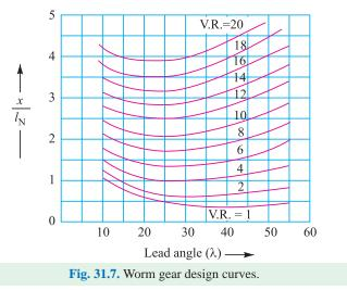
Note : The lowest point on the curve may be determined mathematically by differentiating the equation (*i*) with respect to  $\lambda$  and equating to zero, *i.e.*
