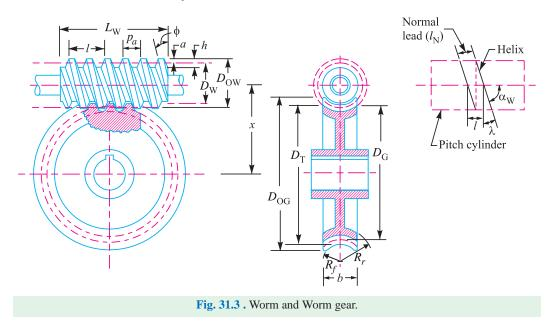
**2.** *Lead.* It is the linear distance through which a point on a thread moves ahead in one revolution of the worm. For single start threads, lead is equal to the axial pitch, but for multiple start threads, lead is equal to the product of axial pitch and number of starts. Mathematically,
