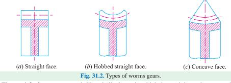
The *straight face worm gear* is like a helical gear in which the straight teeth are cut with a form cutter. Since it has only point contact with the worm thread, therefore it is used for light service.
