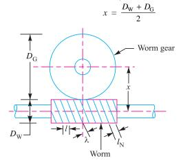
Fig. 31.6. Worm and worm gear.
