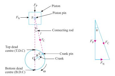
Fig. 32.10. Forces on the connecting rod.
