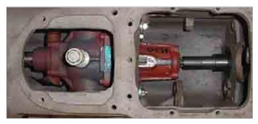
Hydrostatic transmission inside a tractor engine
