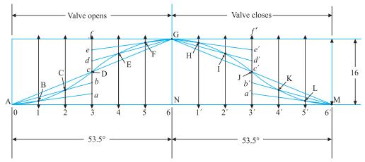
Fig. 32.32. Displacement diagram.
