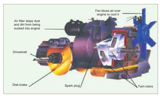
German engineer Fleix Wankel (1902-88) built a rotary engine in 1957. A triangular piston turns inside a chamber through the combustion cycle.
