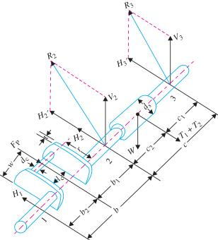
Fig. 32.16. Centre crankshaft at dead centre.
