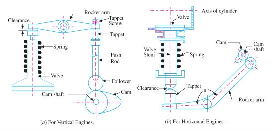
Fig. 32.20. Valve gear mechanism.
