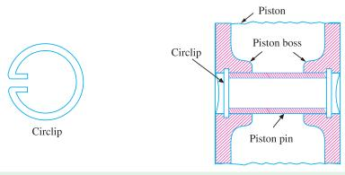
Fig. 32.6. Full floating type piston pin.
