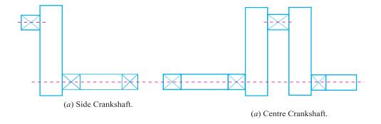
Fig. 32.15. Types of crankshafts.
