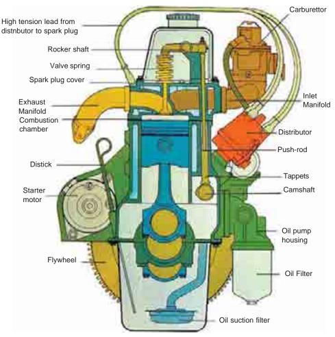
Schematic of a 4 cylinder IC engine
