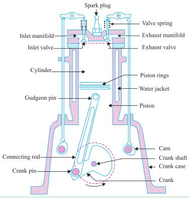
Fig. 32.1. Internal combustion engine parts.
