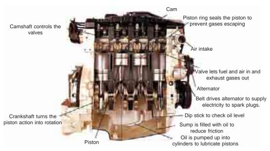
The above picture shows crankshaft, pistons and cylinder of a 4-stroke petrol engine.
