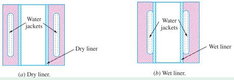
Fig. 32.2. Dry and wet liner.
