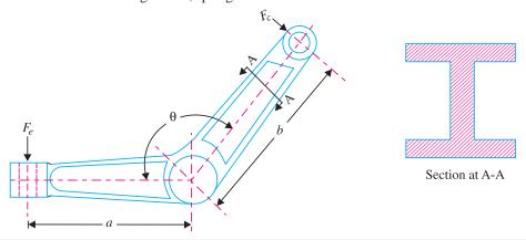
Fig. 32.24. Rocker arm for exhaust valve.
