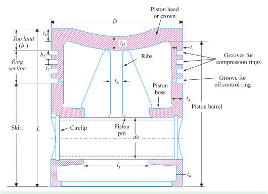
Fig. 32.3. Piston for I.C. engines (Trunk type).
