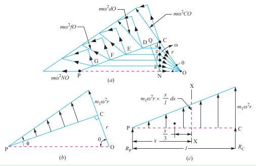
Fig. 32.11. Inertia bending forces.
