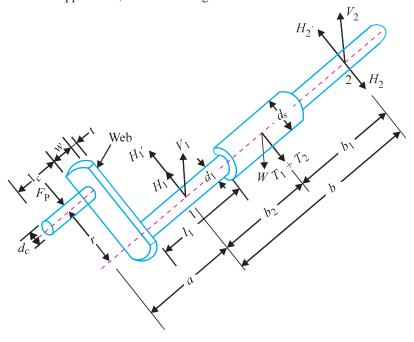
Fig. 32.18. Side crankshaft at dead centre.
