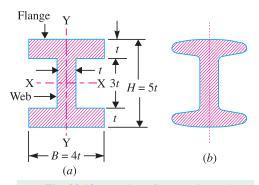
Fig. 32.13. *I*-section of connecting rod.
