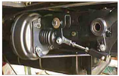
Power-brake mechanism of an automobile
