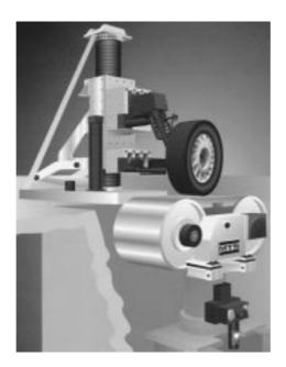
**FIGURE 1.1.1** Artist's concept of a moving stainless steel roadway to drive the suspension system through a spinning, articulated wheel, simulating three-dimensional motions and forces. (MTS Systems Corp., Minneapolis, MN. With permission.) Notes: Flat-Trac<sup>®</sup> Roadway Simulator, R&D100 Award-winning system in 1993. See also Color Plate 1.\*
