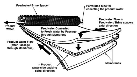
FIGURE 20.6.8 A spiral-wound RO membrane element.
