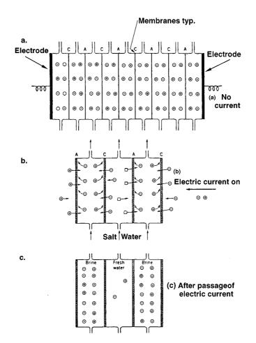
**FIGURE 20.6.10** The ED process. *C* and *A* are cation- and anion-permeable membranes, respectively. Application of electric current causes ion transport in a way that salt is depleted in alternate compartments, and enriched in the remaining ones.
