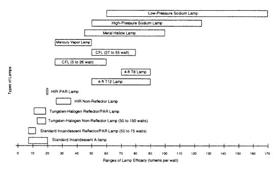
**FIGURE 20.8.1** Ranges of lamp efficacy. (Ballast losses are included for all discharge lamps.) (Compiled from U.S. DOE, 1993a; Morse, personal communication, 1994; and manufacturer's catalogs.)
