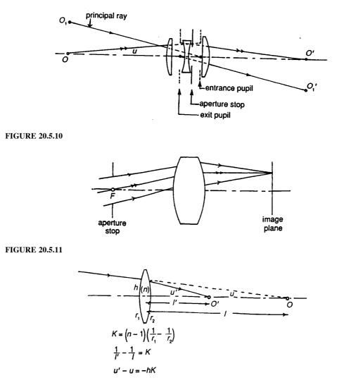
lenses of negligible thickness instead of individual surfaces. Figure 20.5.12 shows the properties of a thin lens. A system of thin lenses can be ray traced to find its properties, locate foci and ray clearances, etc., and very often the results will be good enough to use without further refinement. This is particularly true of systems involving unexpanded laser beams, where the beam diameters are quite small.
