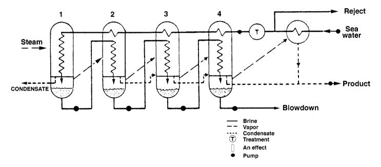
FIGURE 20.6.4 Simplified schematic flow diagram of a typical four-effect VTE desalination plant.
