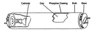
**FIGURE 20.8.2** Typical full-size fluorescent lamp. (From Atkinson, B. et al., *Analysis of Federal Policy Options for Improving U.S. Lighting Energy Efficiency: Commercial and Residential Buildings*, Lawrence Berkeley National Laboratory, Berkeley, CA, 1992. With permission.)
