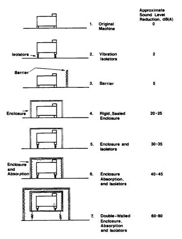
FIGURE 20.7.6 Approximate A-weighted sound level reductions expected from different noise control approaches.
