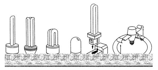
**FIGURE 20.8.3** A variety of compact fluorescent and circular lamps: (a) twin-tube integral, (b and c) triple-tube integrals, (d) integral model with glare-reducing casing, (e) modular quad tube and ballast, and (f) modular circline and ballast. (Courtesy of Katherine Falk and *Home Energy* magazine, 1995.)
