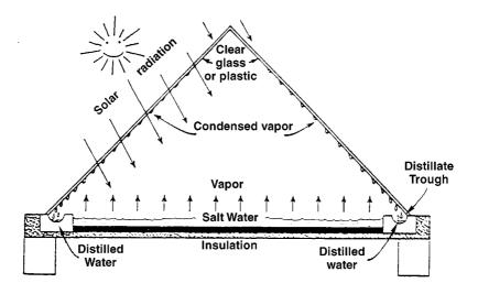
FIGURE 20.6.7 A typical basin-type solar still.
