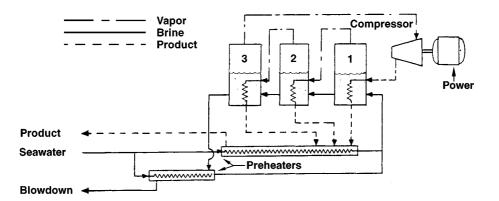
FIGURE 20.6.6 Schematic flow diagram of a ME vapor compression submerged-tube desalinaton plant with three effects.
