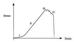
FIGURE 20.3.2 General stress-strain behavior of connective soft tissue.
