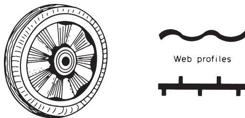
Fig. 28.14. A design for a small plastic wheel. The upper, corrugated, web profile is better than the lower, ribbed, one because the section is constant.
