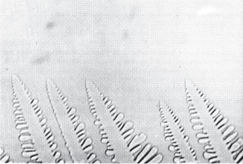
Fig. 6.8. Most metals solidify with a dendritic structure. It is hard to see dendrites growing in metals but they can be seen very easily in transparent organic compounds like camphene which – because they have spherical molecules – solidify just like metals.
