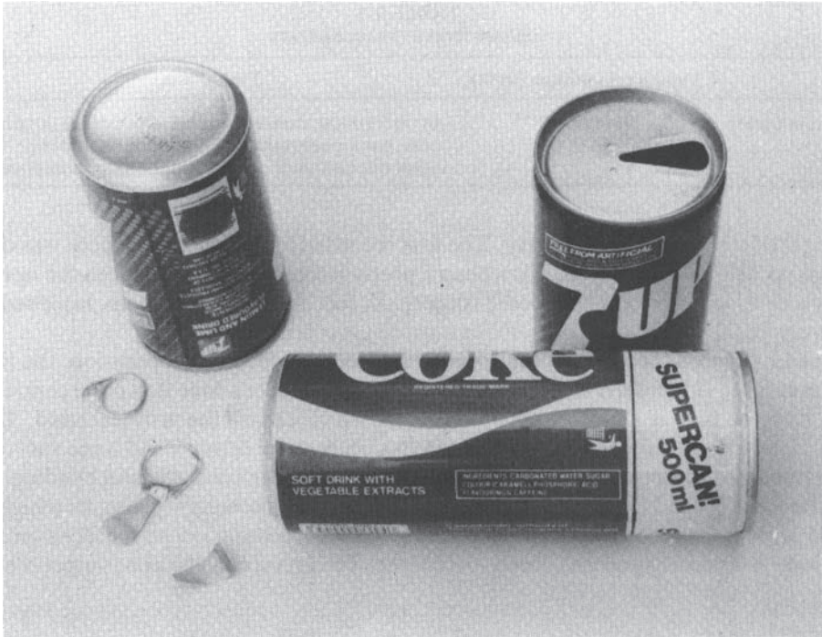
Fig. 1.5. The aluminium drink can is an innovative product. The body is made from a single slug of a 3000 series aluminium alloy. The can top is a separate pressing which is fastened to the body by a rolled seam once the can has been filled. There are limits to one-piece construction.
