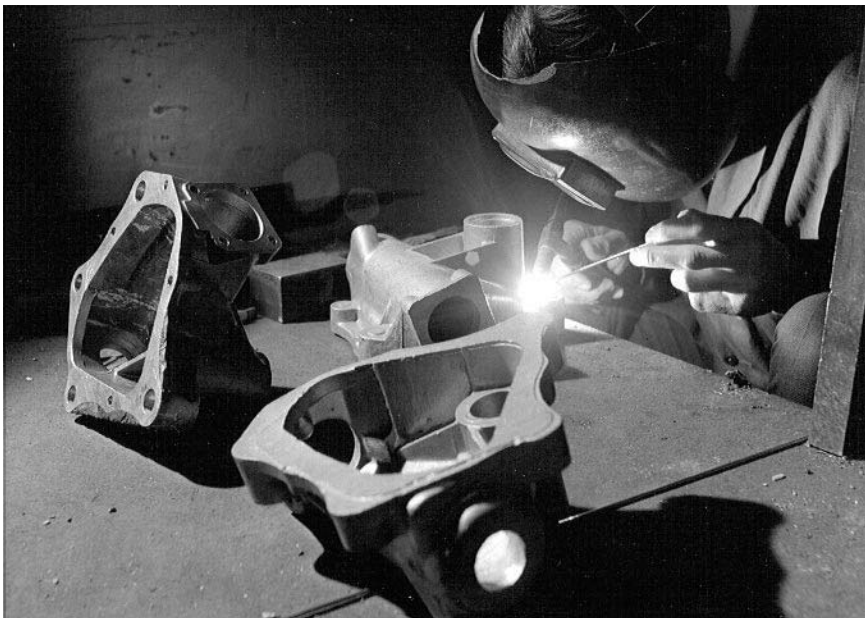
3.4 Tungsten inert gas welding (photograph by courtesy of TWI).
