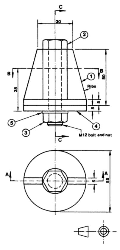
Fig 10.2 Outside bracket assembly
