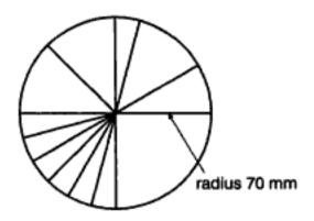
Fig 1.9 Drawing lines at different angles
