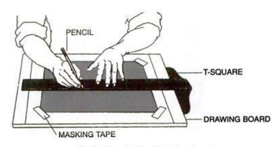
Fig 1.2 An A3-size drawing board
