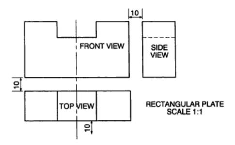
Fig 3.4d For three views of an object
