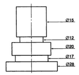
Fig 3.11 Dimensioning of diameters placed outside component
