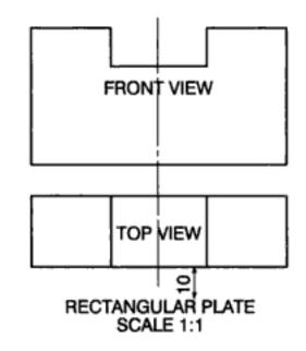
Fig 3.4b For two views of an object
