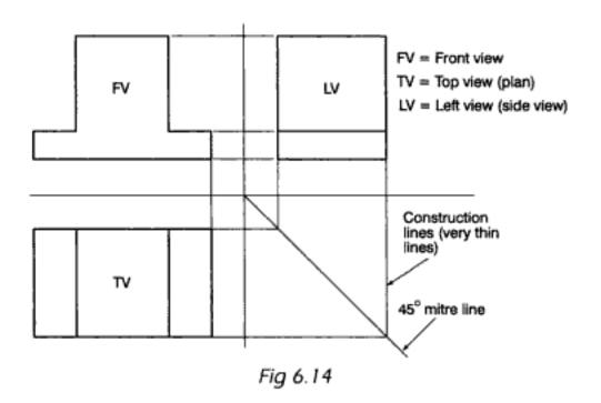
Two views of an object are given in first-angle orthographic projection. Construct the two given views and find the third view, as explained in fig 6.14. Scale 1:1.
