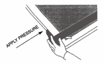
Fig 1.4 Apply pressure to the side of the T-square. Keep pressing towards the right to keep the T-square tightly secured to the edge of the drawing board
