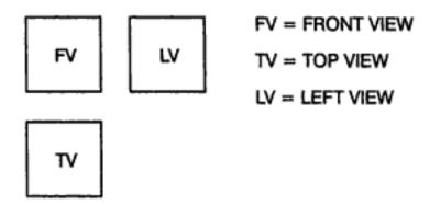
3 In third-angle orthographic projection, you see three separate views, but the arrangement of the views is different as shown below.
