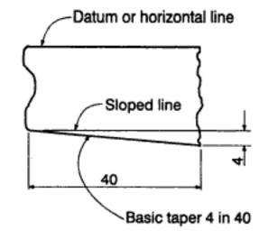
Fig 3.14c Dimensioning a taper (basic)
