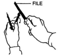
Fig 1.17 Sharpening your compass lead with a file
