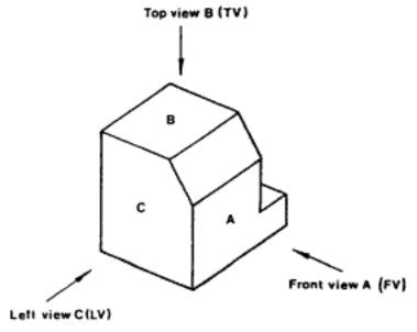
Fig 6.3 Isometric view
