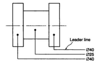
Fig 2.7b Leader lines terminating in a dot (limited space)
