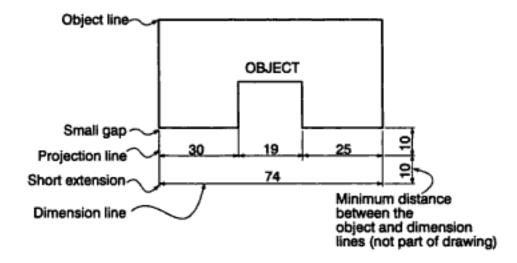
Fig 3.5a Dimensions below the view of an object
