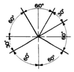
Fig 3.7c Orientation of angular dimensions
