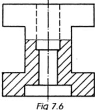
Where an area of hatching touches the centre line, the centre line must be changed to a continuous 0,3 mm thick line.
