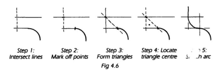
To draw an arc between two curved lines, use the same construction as for the two previous examples.
