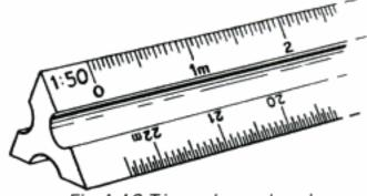
Fig 1.19 Triangular scale rule
