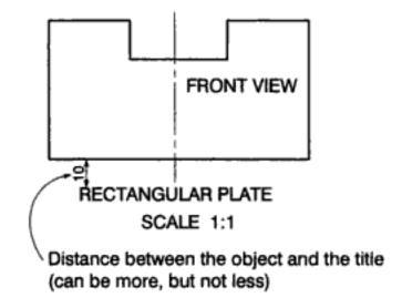
Fig 3.4a For a single view of an object
