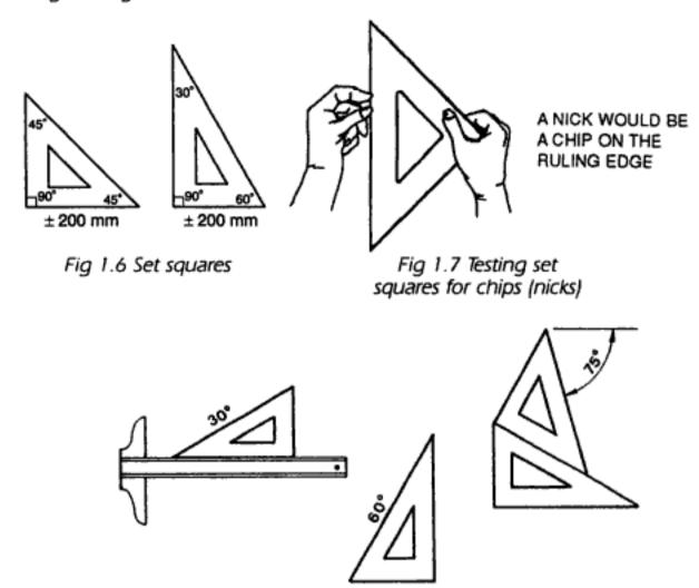
Fig 1.8 Drawing different angles using the set squares
