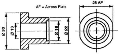
Fig 3.10 Arrangement of dimensioning of diameters
