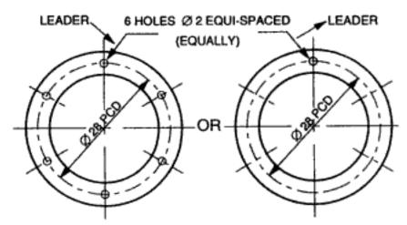
Fig 3.12 Holes on a pitch circle by using leaders
