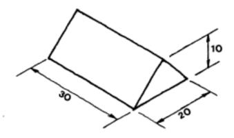
Fig 4.24 Part to be drawn isometrically
