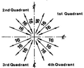
Fig 3.7b Orientation of inclined linear dimensions
