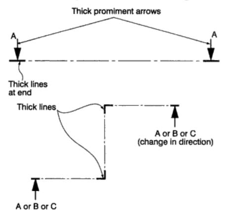
Fig 2.12a Cutting planes or sectional planes (Line type H)
