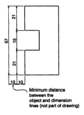
Fig 3.5c Dimensions to the left of the view of an object
