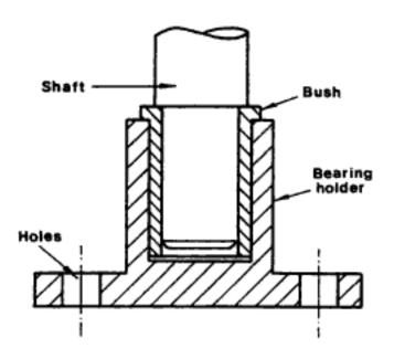
Fig 10.1 Sectional assembly drawing of a shaft, bush and bearing holder
