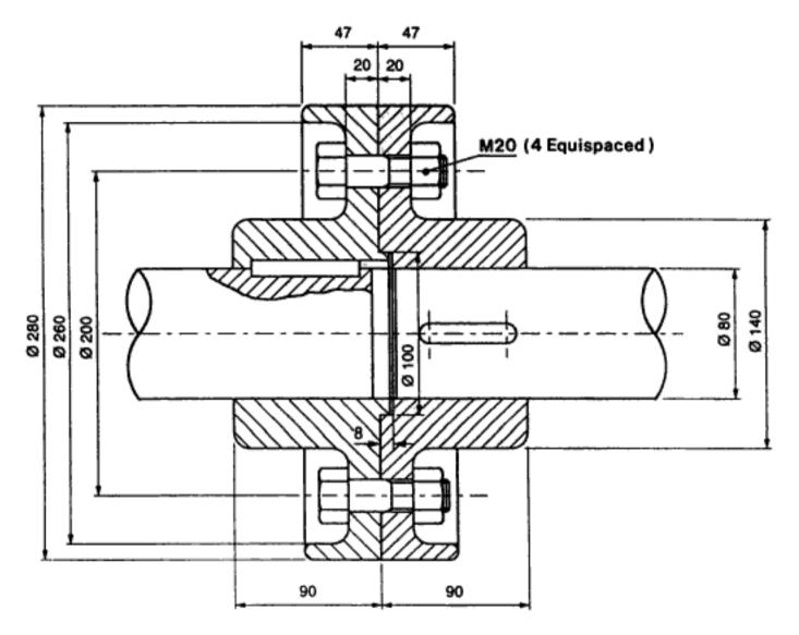
Fig 10.5 A flange-coupling in section
