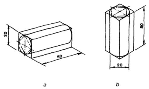
Fig 4.27a-b Isometric sketch of a round bar
