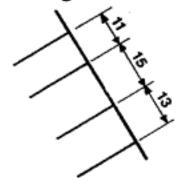
Fig 3.7a Linear dimensions are written parallel to the dimension line
