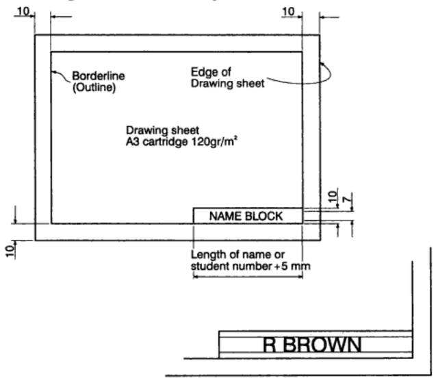
Fig 3.1 Preparation of the drawing sheet
