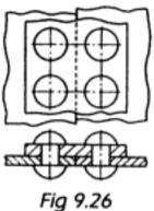
Double-riveted butt joint with a double cover plate (zigzag-riveted)
