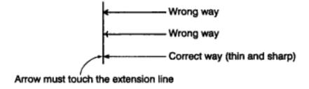
Fig 3.5d The correct and incorrect ways of inserting arrowheads
