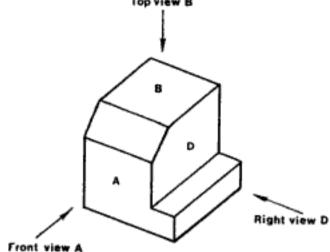
Fig 6.5 The arrows perpendicular (at right angles) to the faces or planes
