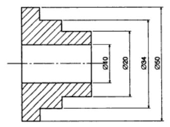
Fig 3.9 Dimensioning of diameters (side view)
