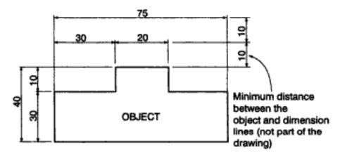
Fig 3.5b Dimensions above the view of an object
