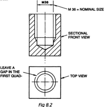
Fig 8.3 shows the different angles and measurements needed to draw a representation of a metric thread and the drilled hole. The nominal size of the metric thread is the bigger diameter and the diameter is  $0.8 \times \text{nominal size}$  (M36) in millimetres.
