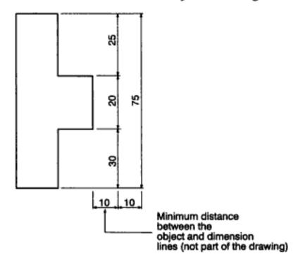
Fig 3.5e Dimensions to the right of the view of an object
