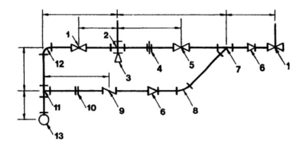
Fig. 11.3 Former single-line drawing symbols which are sometimes still used
